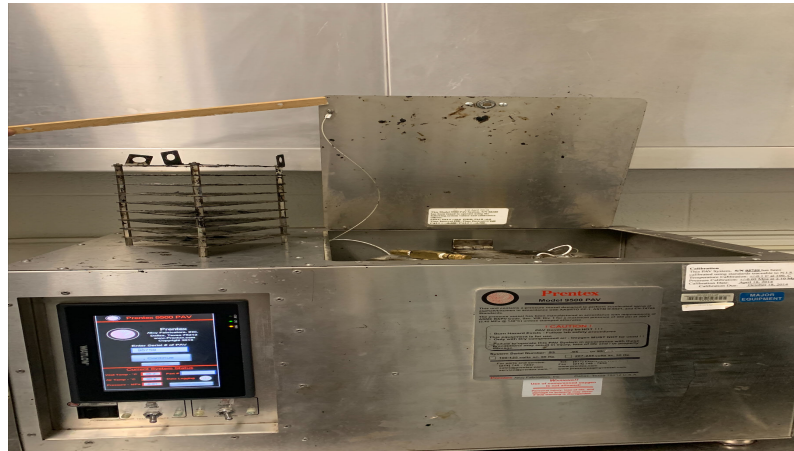
Figure 3.5: Pressurized Aging Vessel (PAV)
