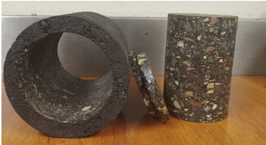
Figure 3.10: Test Specimen after Cutting and Coring.
