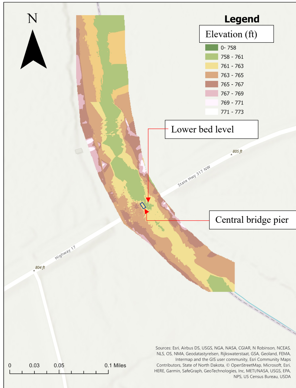
Figure 7. Bathymetry of the study site at Highway 17 Bridge near Grafton.
