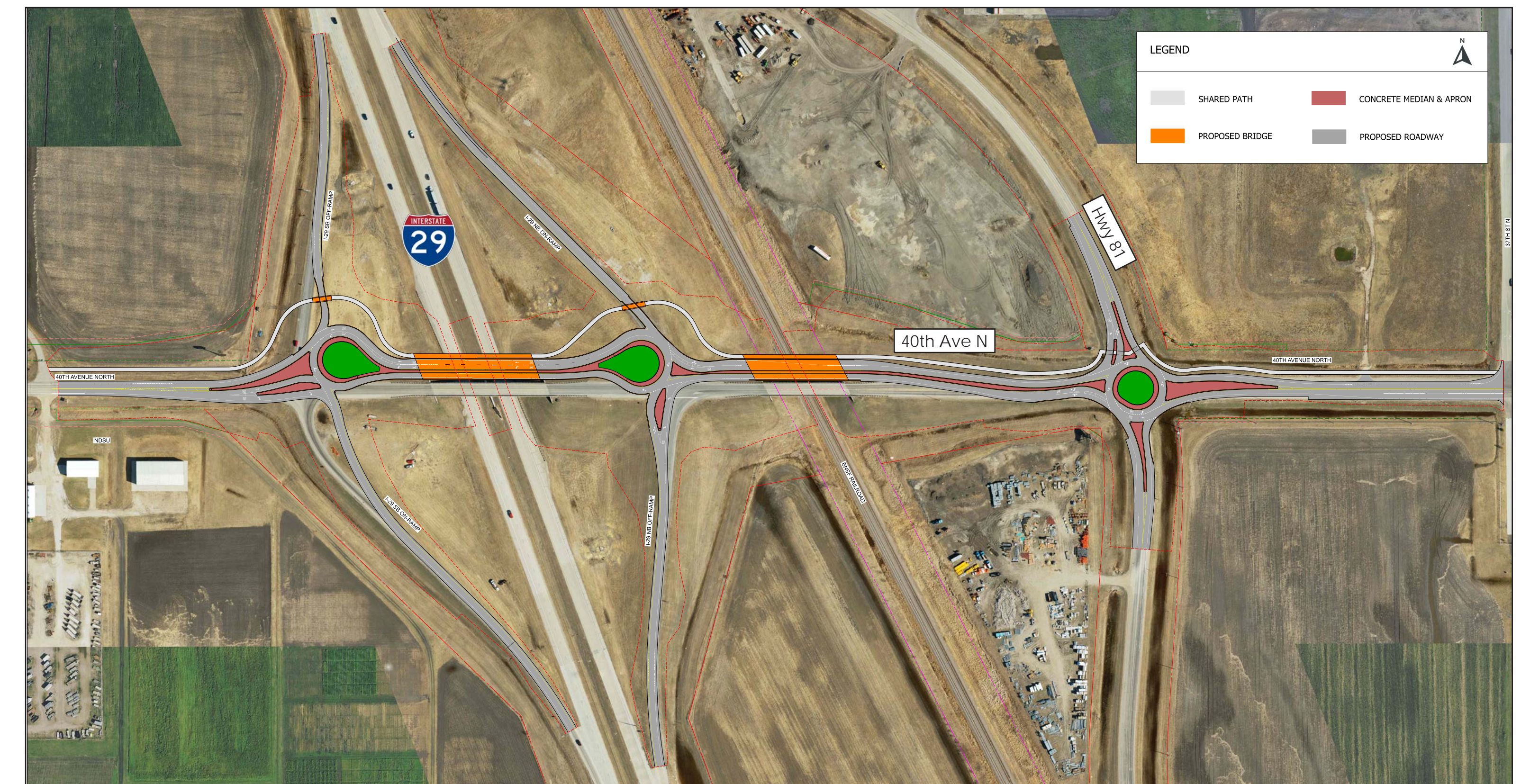
Dumbbell interchange identified as the alternative to advance to the next phase of project development.
