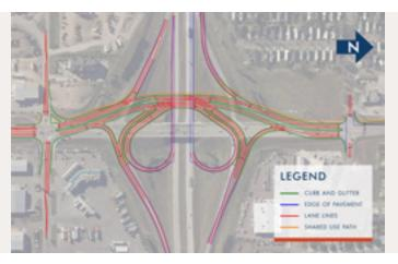
The North Dakota Department of Transportation has selected alternative four, a modified single-point urban interchange (SPUI), from five proposed options for reconstruction of the I-94 Interchange (Exit 161) in the summer of 2024.
