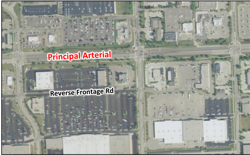
Development with Reverse Frontage and Limited Access onto the Principal Arterial, DO THIS
