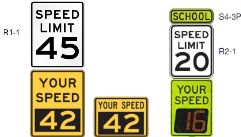
6. The changeable portion of the VSFS legend should be the same height, width, and stroke of those on the Speed Limit sign it supplements or is mounted below.
