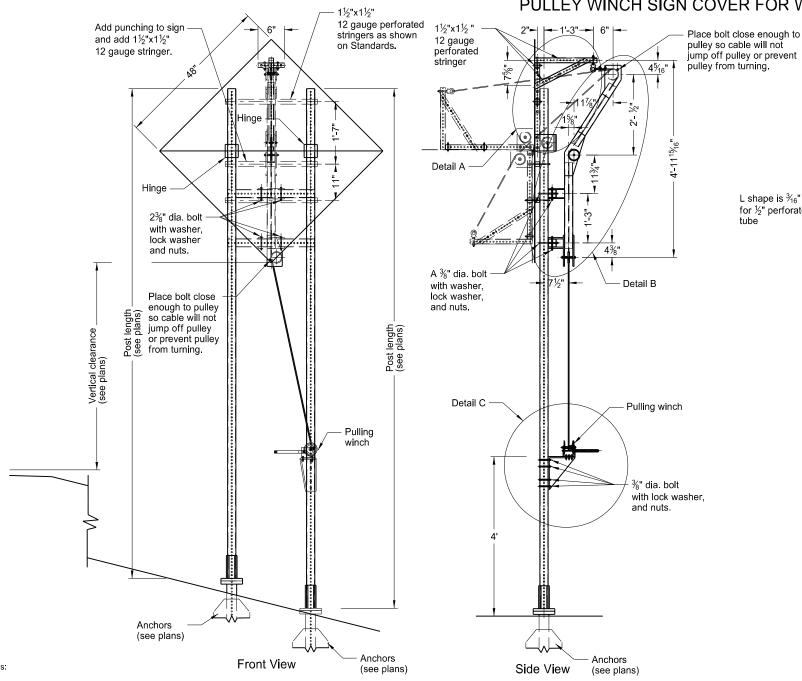
A %" dia. forged or machine eye bolt with shoulder, washer, lock washer, and two nuts. 12 gauge perforated stringers as shown on Standards. Front View **├--** 6½" <del>- |</del> Side View
