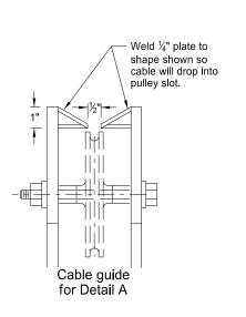
$\frac{1}{4}$ " dia. bolt with washer and lock washer and nut with spacer to prevent the freewheeling of the pulley. 1/4" dia. bolt with washer and lock washer and nut with spacer to prevent the freewheeling of the pulley. Side View
