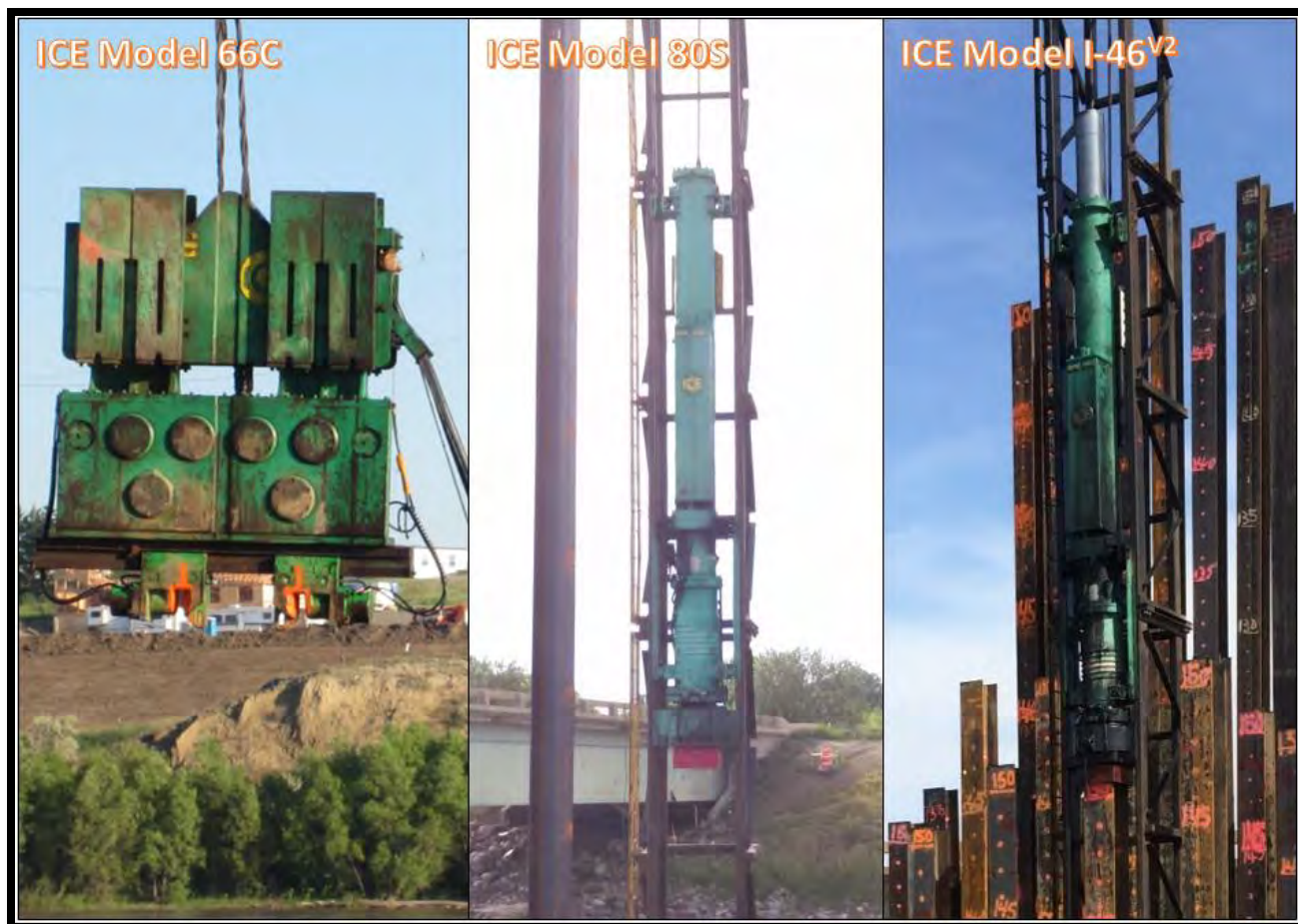
Figure 3, Vibratory and Impact Hammers
