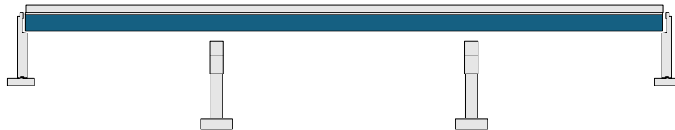
Balanced Span Arrangement
