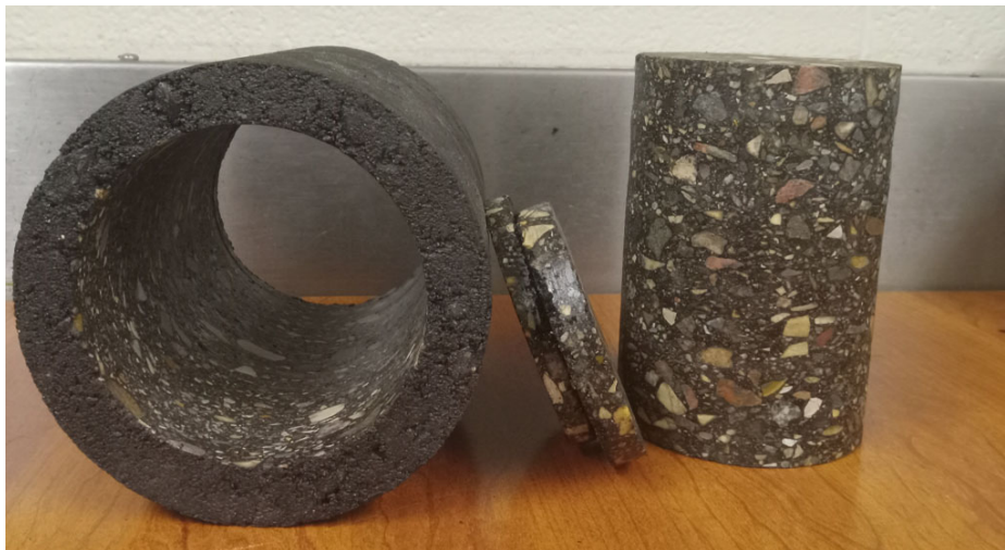
Figure 3.10: Test Specimen after Cutting and Coring.
