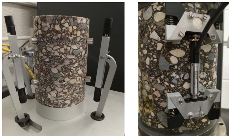
Figure 3.13: Mounting Studs on Test specimen and LVDT Attached to Holding Brackets
