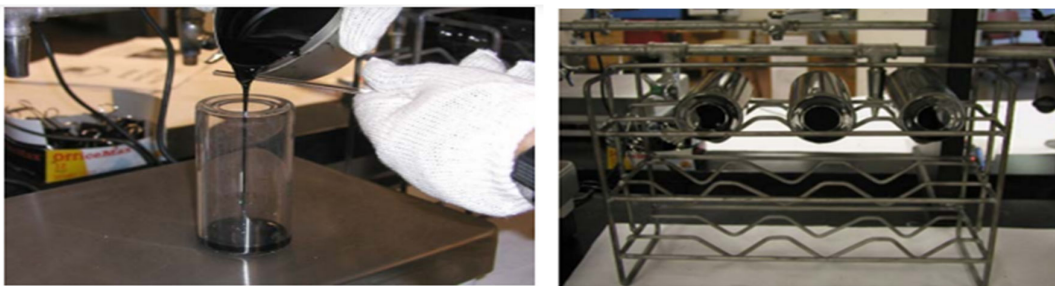
Figure 3.4: Pouring 35 \pm 0.5 g of Binder into each Container and Container Cooling on Sample Rack
