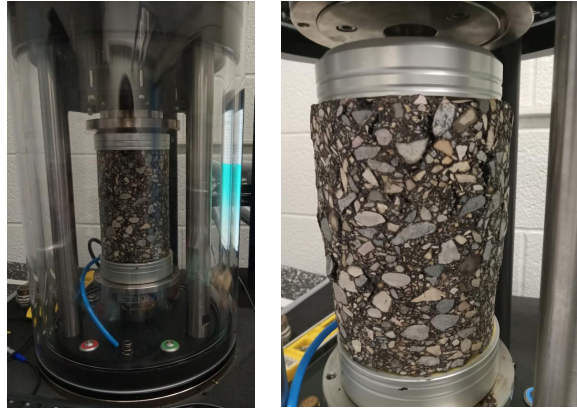
Figure 3.14: Specimen before and after F_N Test
