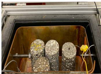
Figure 3.12: Test Specimens with Dummy Specimen Before Temperature Conditioning.
