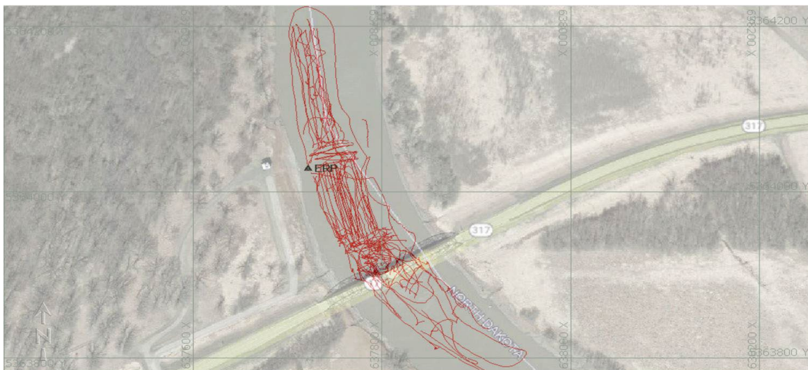
Figure 5. HYCAT's autonomous route at the site of Highway 17 Bridge near Grafton.
