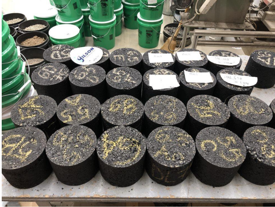
Figure 16. Asphalt Samples Ready for G_{sb} Experiment
