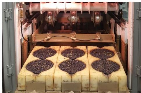
Figure 4. Asphalt Pavement Analyzer
