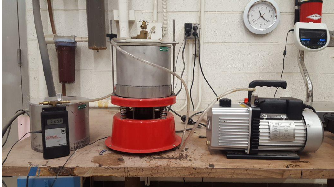
Figure 12. Theoretical Maximum Specific Gravity ( G_{mm} ) Experiment Set-up
