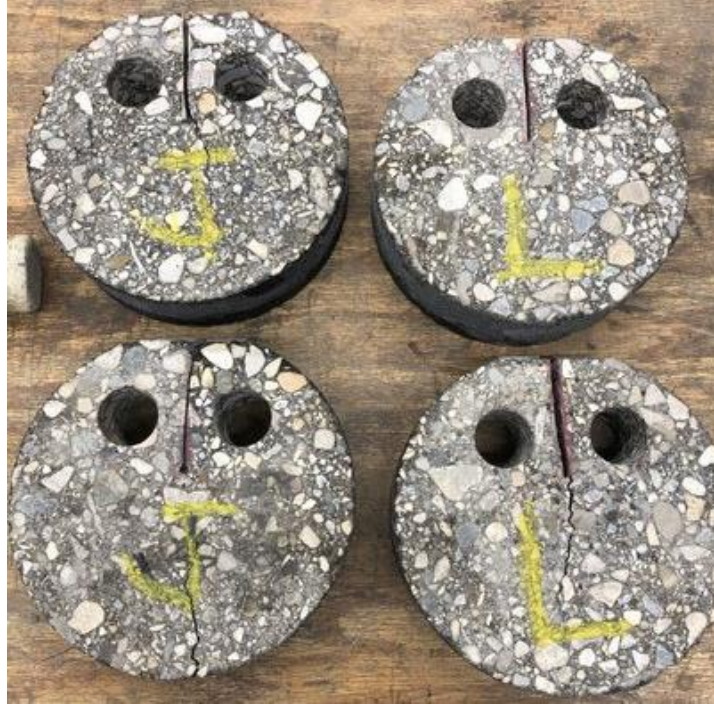
Figure 38. Typical Before and After DCT Test Samples
