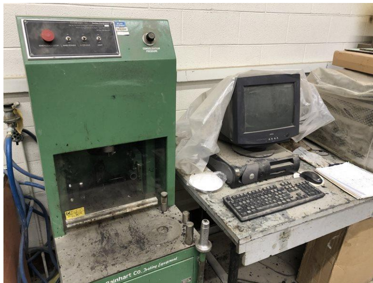
Figure 14. SuperPave Gyrotory Compactor
