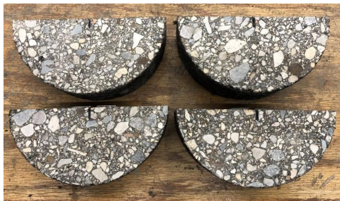
Figure 21. SCB Samples Ready for Testing
