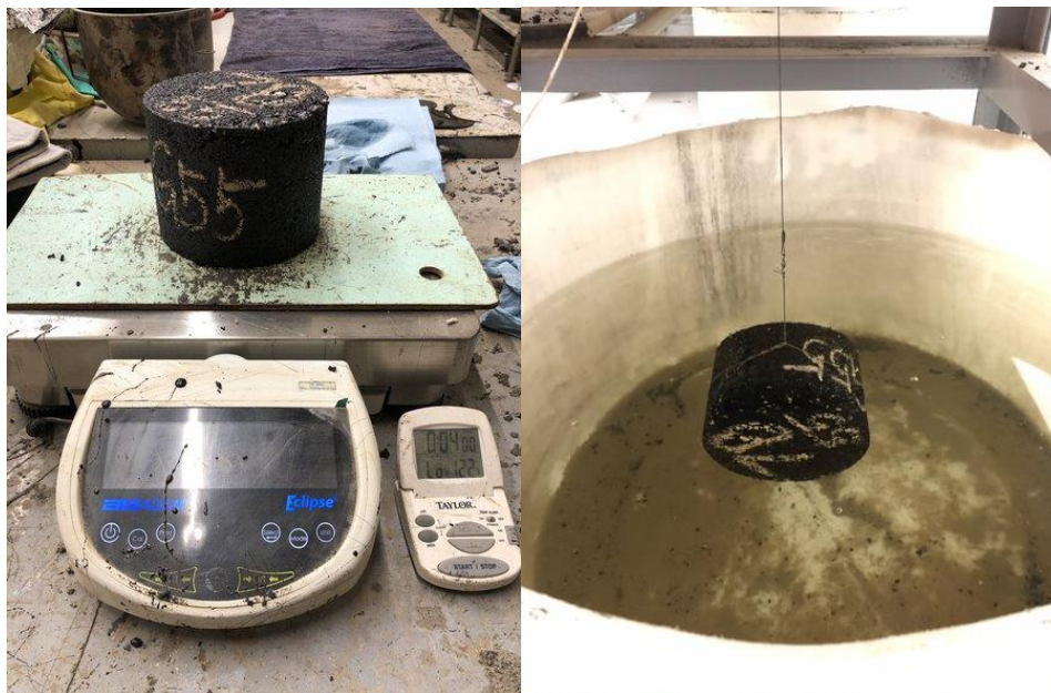
Figure 15. Sample Asphalt Plug Weighed in Air and Sample Submerged Under Water
