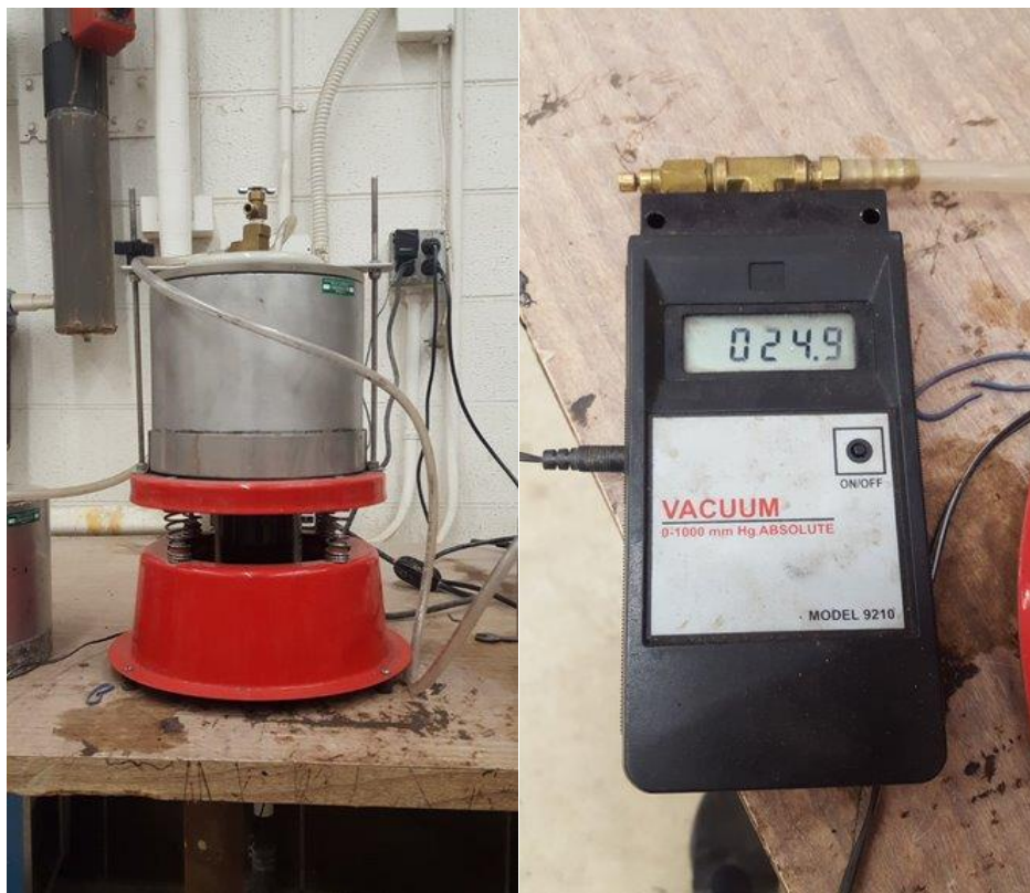
Figure 11. Set-up of bowl and Vacuum Gauge
