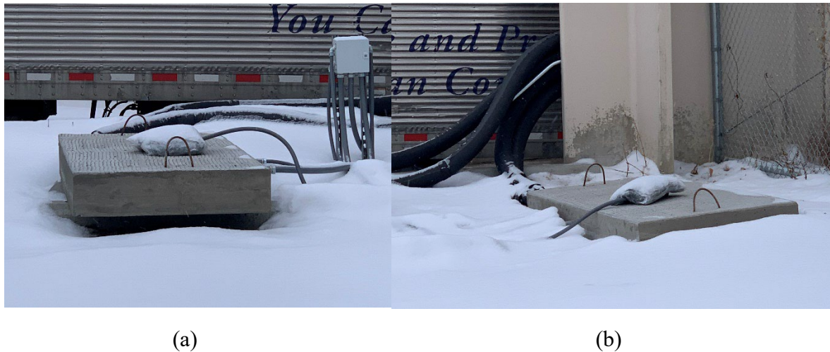
Figure 3.1 Snow-Melting Concrete Panel (a) with rebar, and (b) without rebar
