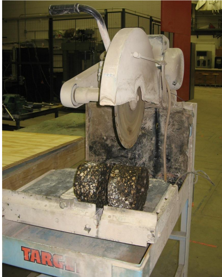
Figure 1: The Saw Used in Sizing the Specimens to APA Height Requirements.
