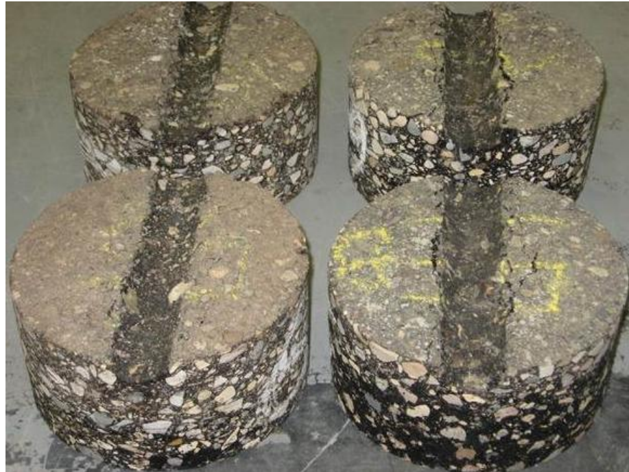
Figure 3: Rut Depths of One APA Run: HMA (left) and WMA (right).
