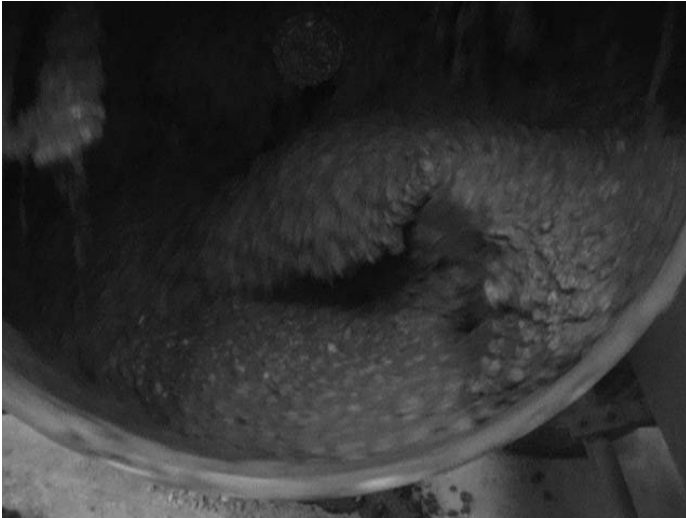
Figure 23: SCC rolling in the mixer
