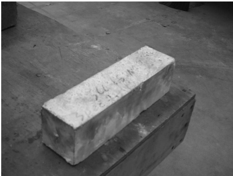
Figure 37: Length change specimen.
