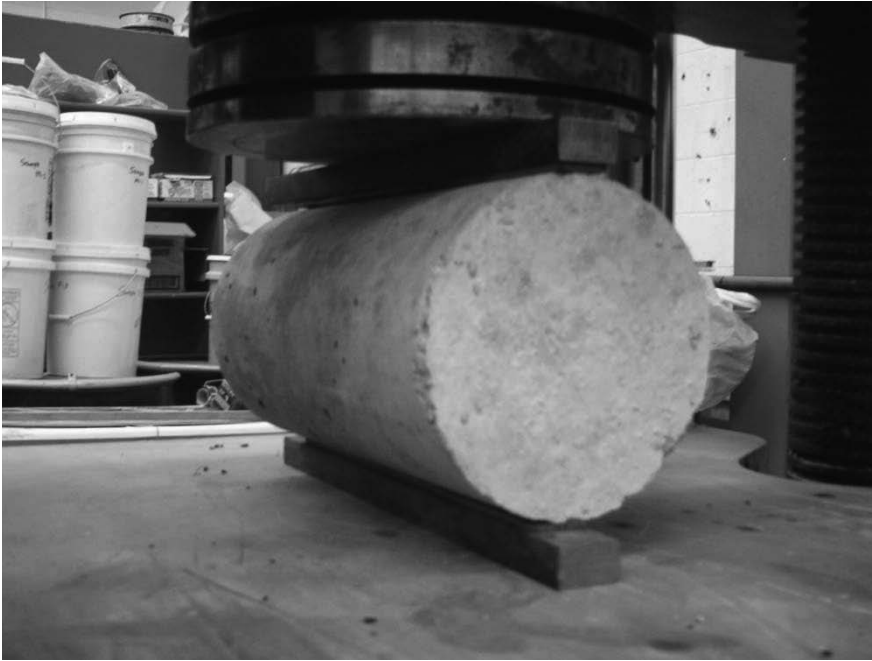
Figure 41: Splitting Tensile Test Setup.
