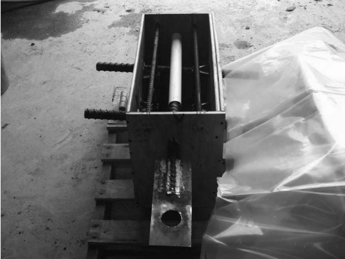
Figure 44: Pullout specimen before casting in concrete
