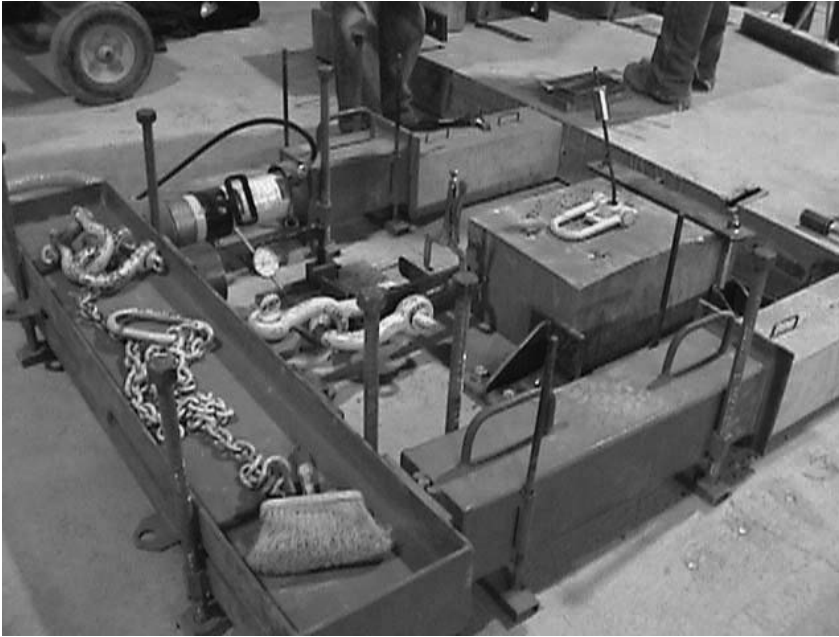
Figure 43: Pullout Test Setup.
