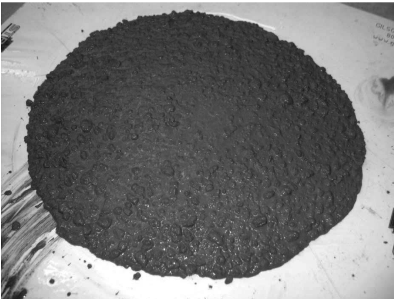
Figure 18: Spread of SCC:6.5:30FA with VSI=0, ideal spread
