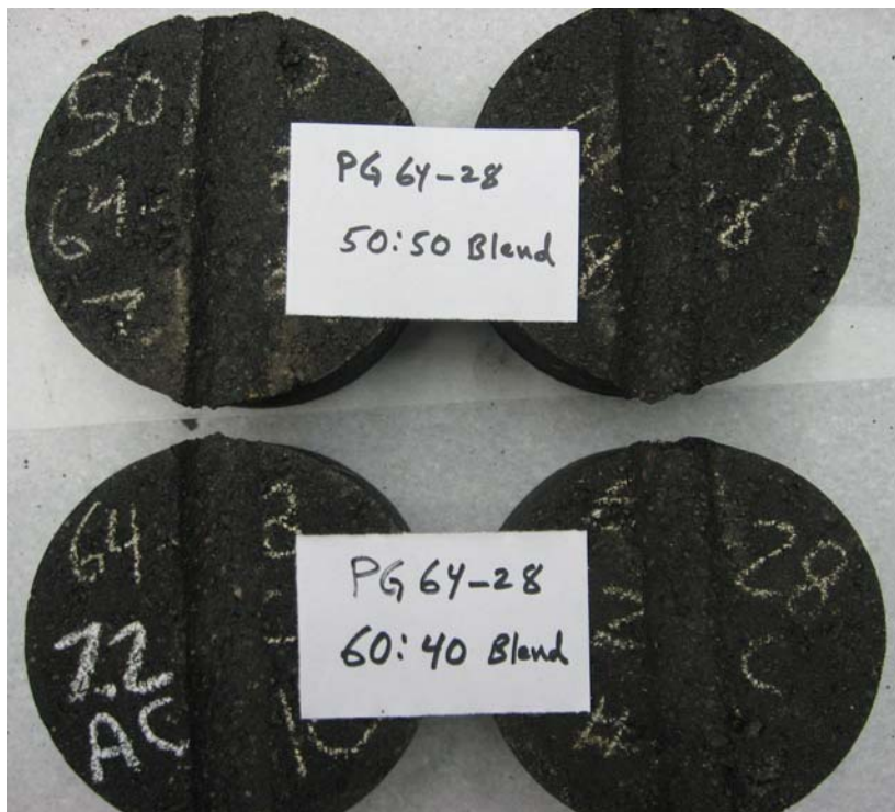
Figure 4 Comparisons between 60:40 and 50:50 Blends in No. 4 Mix with PG 64-28 Binder
