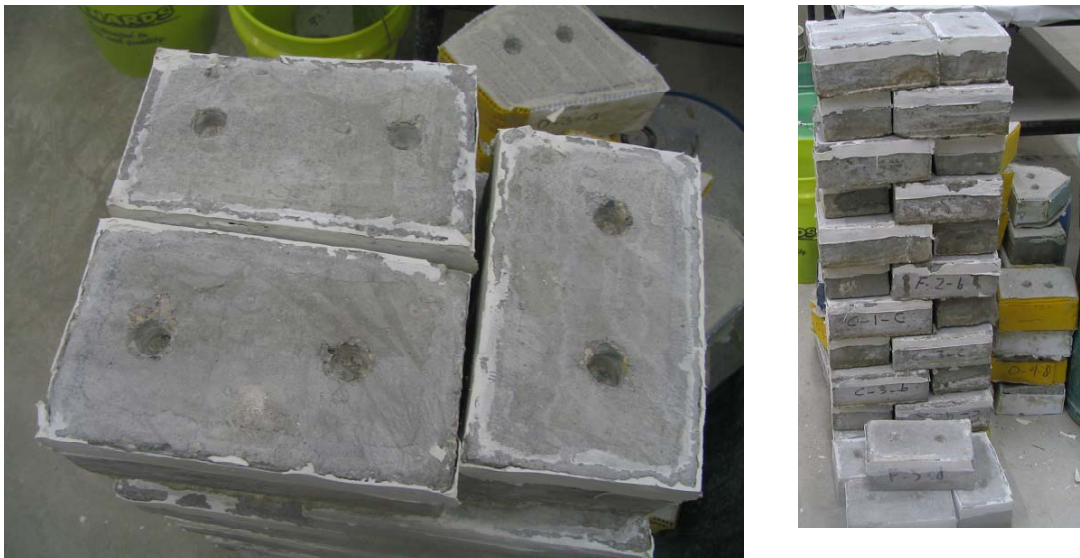
FIGURE 17. Sampling and Testing for Chloride Ion Penetration in Concrete and Concrete Raw Materials: AASHTO T 260-97 Standards.
