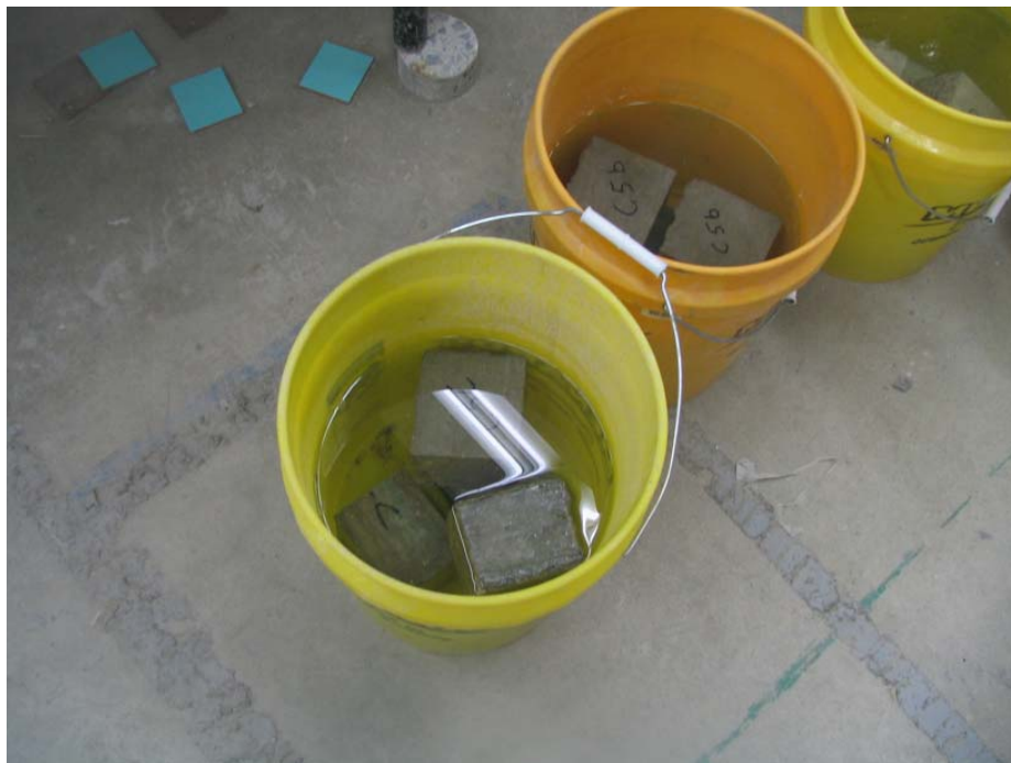
FIGURE 22. Test for Average Depth of Penetration; Specimens in Water.
