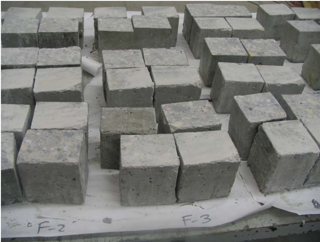
FIGURE 21. Test for Average Depth of Penetration: NDDOT Specifications, Cutting of Each Specimens into Four Pieces.
