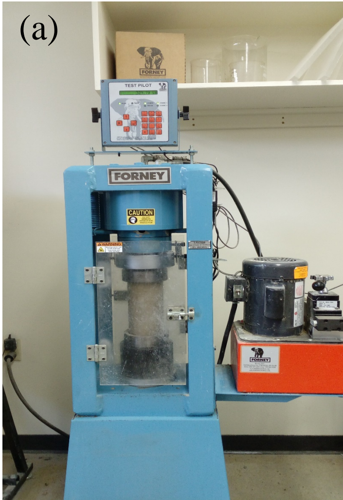
Figure 35 Compressive strength testing scheme (a) and Specimen after failure (b)
