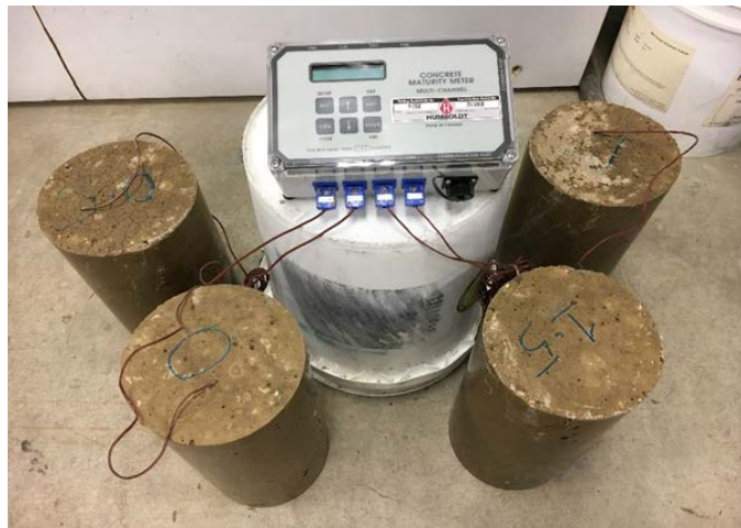
Figure 53 Testing set up for real time maturity measurement
