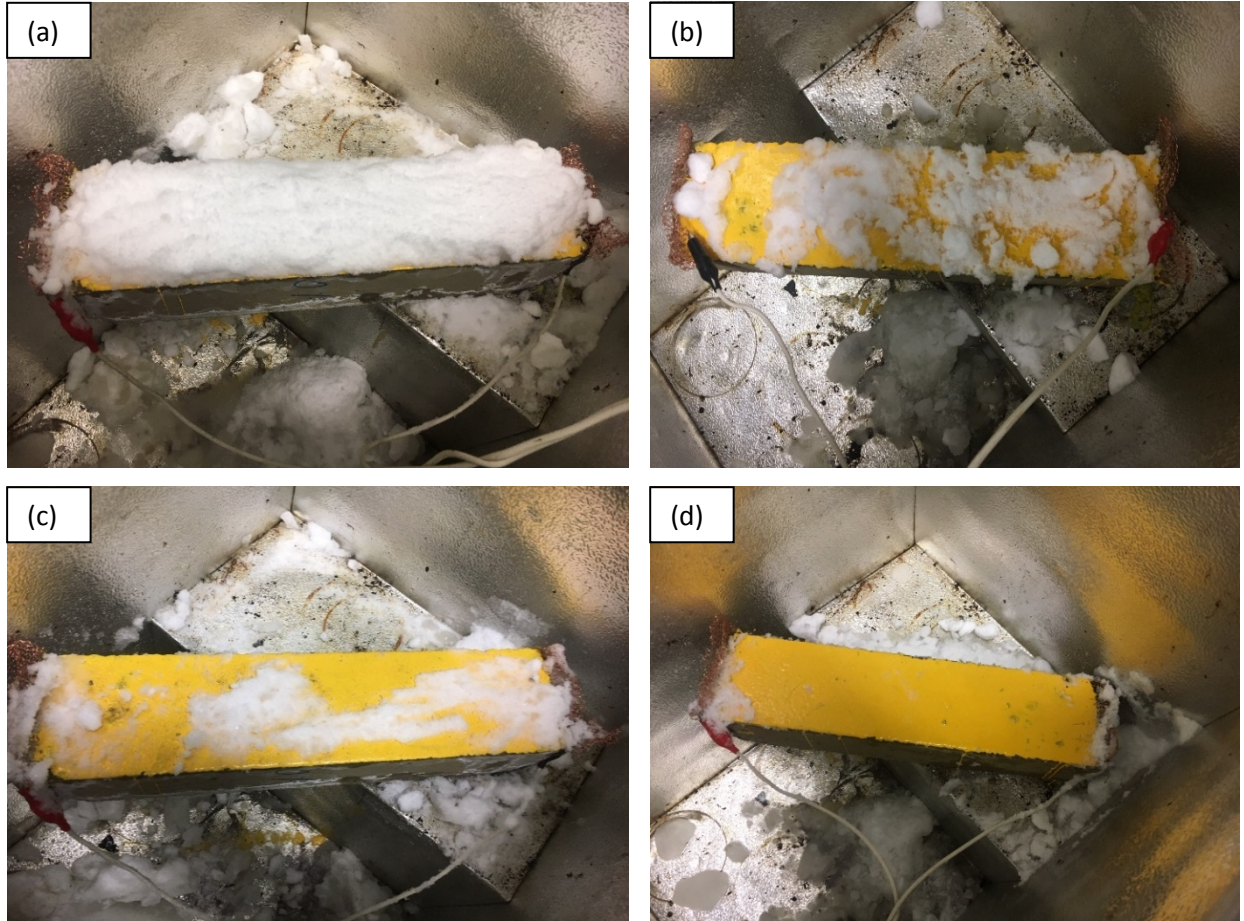
Figure 69 Melting process of Specimen with 1.5 % fiber content for 1.5 inch fluffy snow at -20°C (a) Initial condition, (b) after 40 minutes, (c) after 1 hour 20 minutes, and (d) after 1 hour 35 minutes
