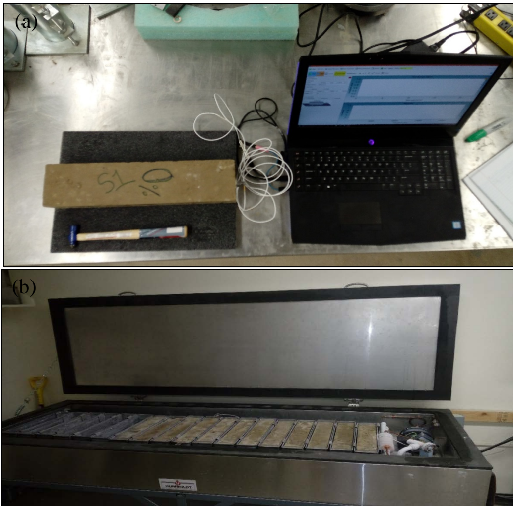
Figure 48 Freeze-thaw chamber (a) and testing scheme of concrete specimen (b)
