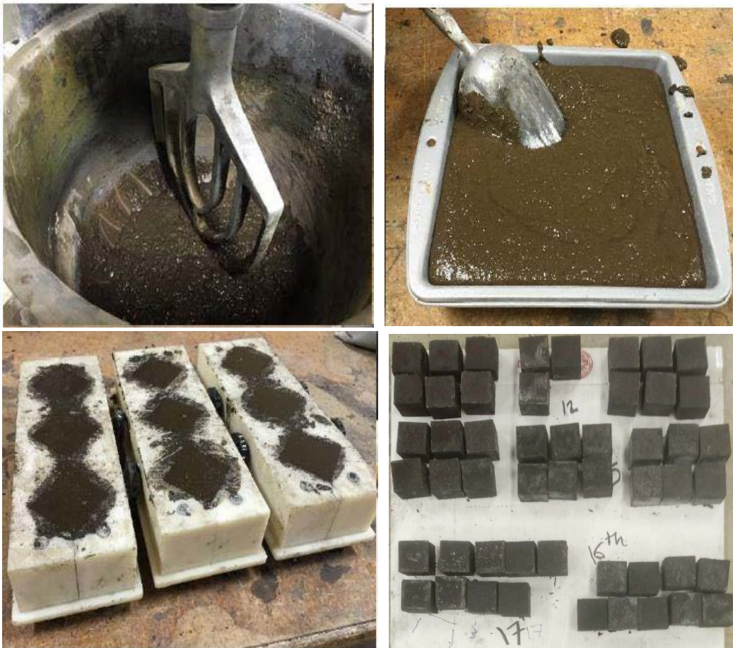
Figure 2 Mixing, molding and demolding
