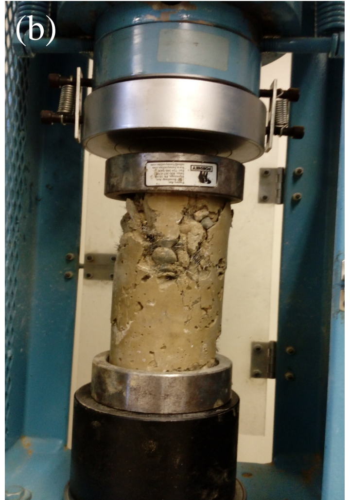
Figure 35 Compressive strength testing scheme (a) and Specimen after failure (b)
