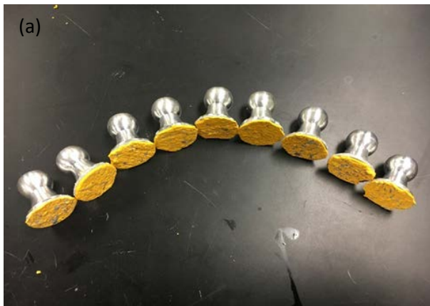
Figure 52 Dollies after pull-off adhesion test; (a) OPC based concrete and (b) Geopolymer concrete
