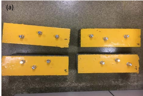
Figure 51 Placing dolly on painted concrete surface (a) and testing instrument set up (b)
