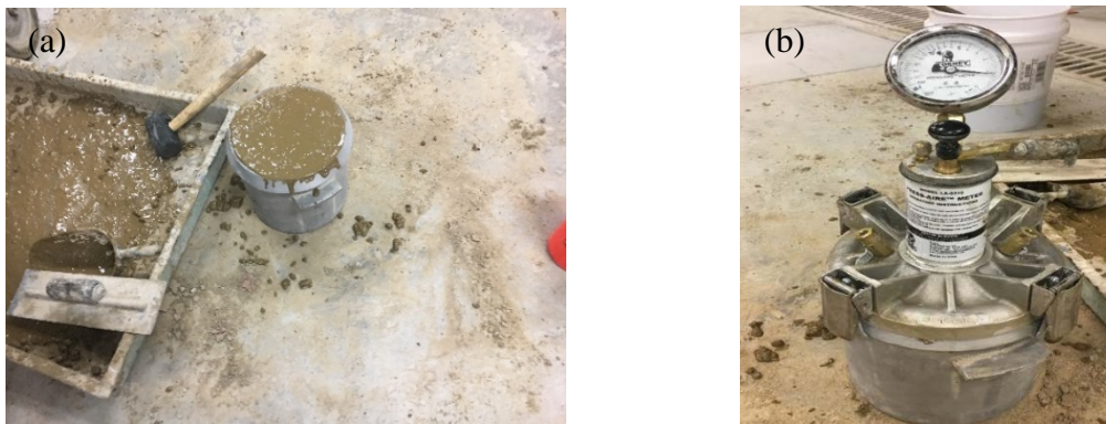
Figure 56 Air content measurement of the fresh geopolymer concrete per ASTM 321, (a) Fill the container of the air meter, (b) Air content measurement result after pressure releasing
