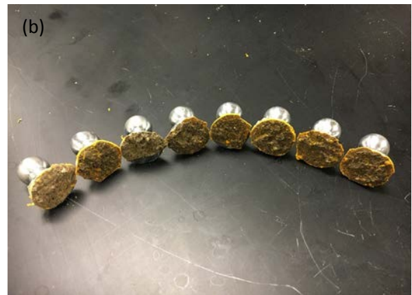
Figure 52 Dollies after pull-off adhesion test; (a) OPC based concrete and (b) Geopolymer concrete
