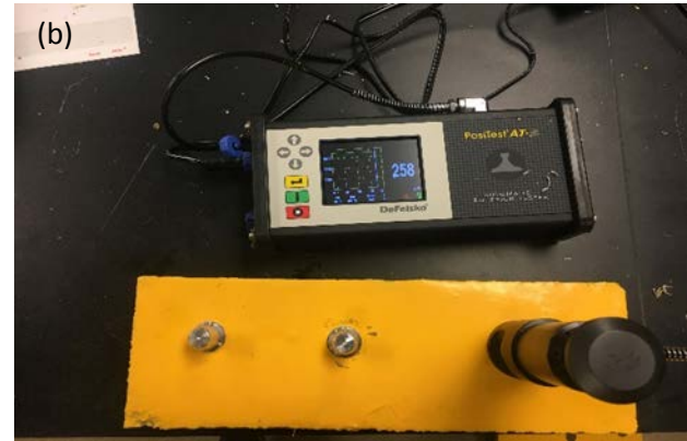
Figure 51 Placing dolly on painted concrete surface (a) and testing instrument set up (b)
