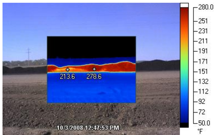
Figure 7. Temperature variations within a windrow of HMA
