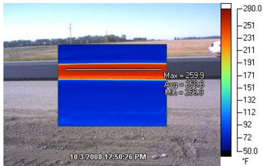
Figure 8. Temperature variations within the asphalt mat placed
