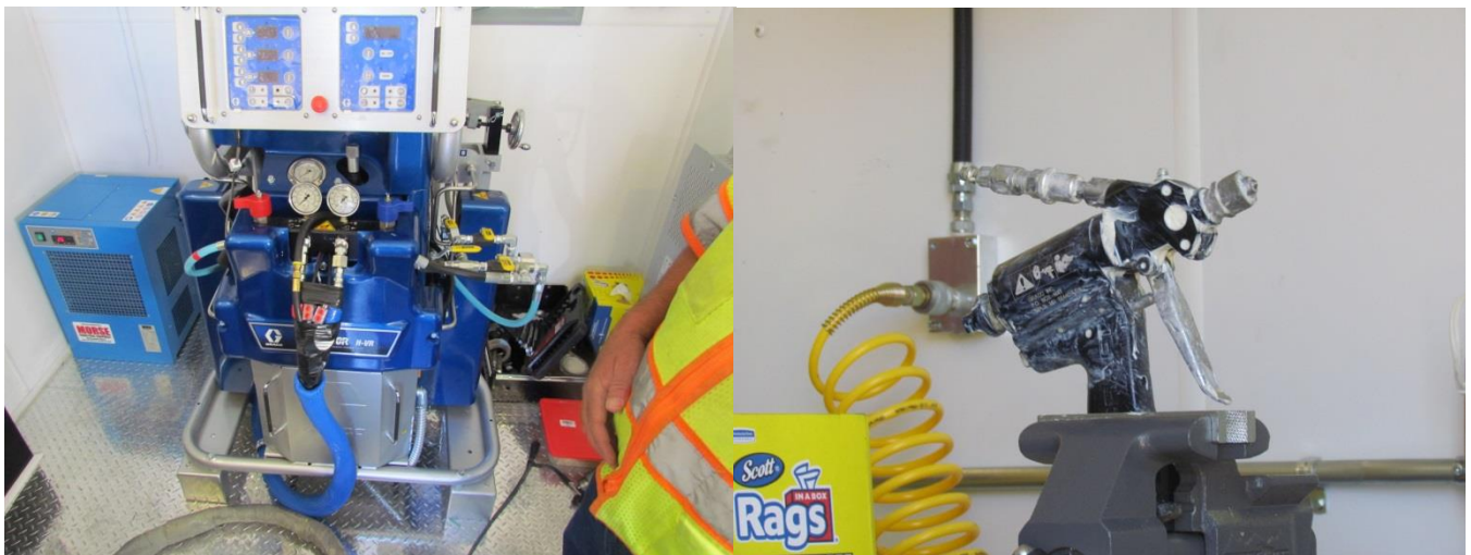
Photo 6 – Pump and spray nozzle used for Spraywall application.
