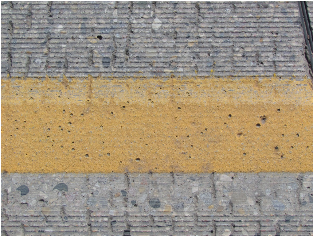
Segment 2B - NB Yellow Grooved Epoxy with 3M AW Elements – RP 143
