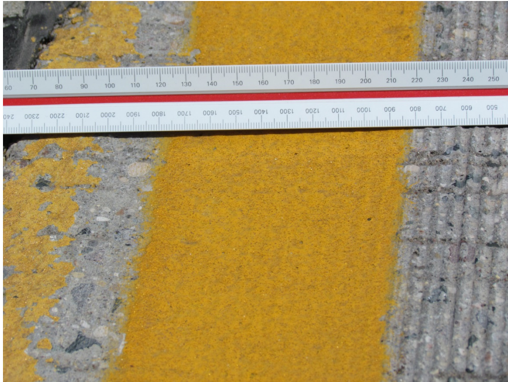
Segment 1A - NB Yellow Grooved Paint with Standard Glass Beads – RP 137
