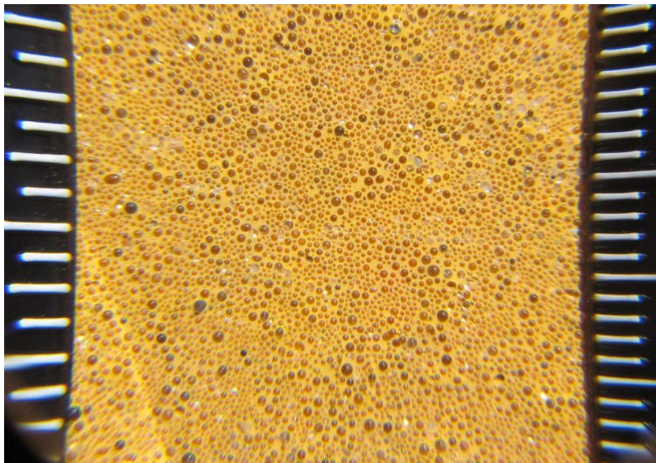
Photo 7: Magnified grooved epoxy with standard glass after 3 winters.
