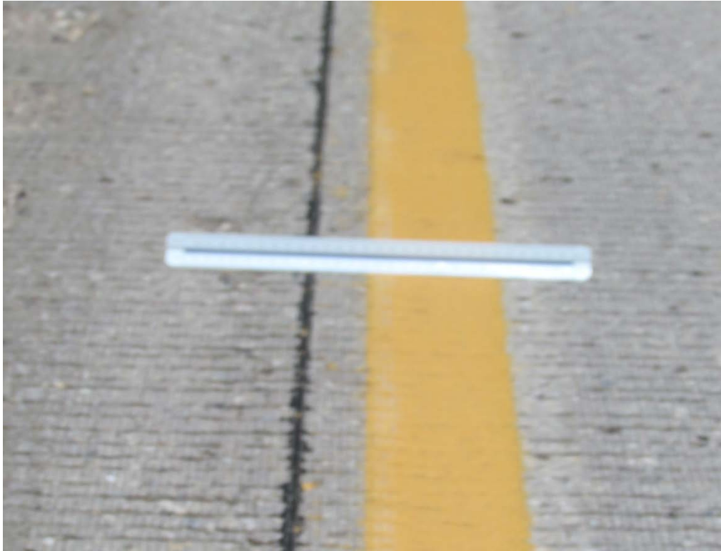
Segment 2A - NB Yellow Grooved Epoxy with Standard Glass Beads – RP 141
