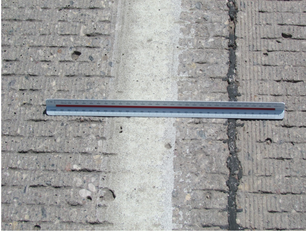
Segment 2A - SB White Grooved Epoxy with Standard Glass Beads – RP 141
