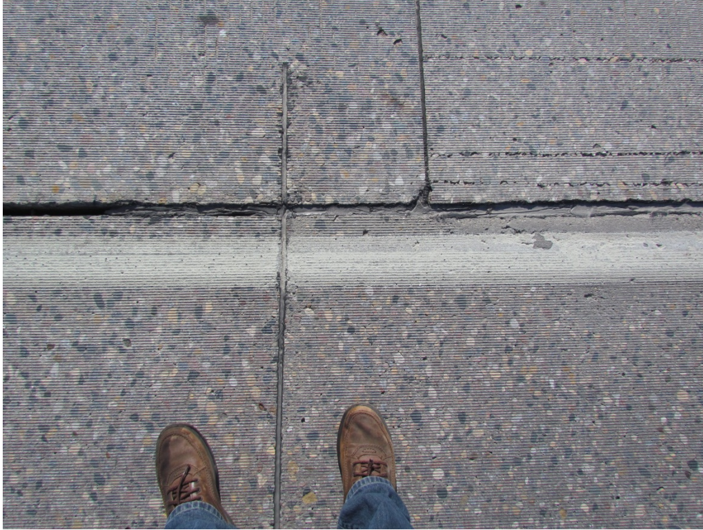
Segment 3A - NB White Surface Applied Epoxy with Standard Glass Beads – RP 145
