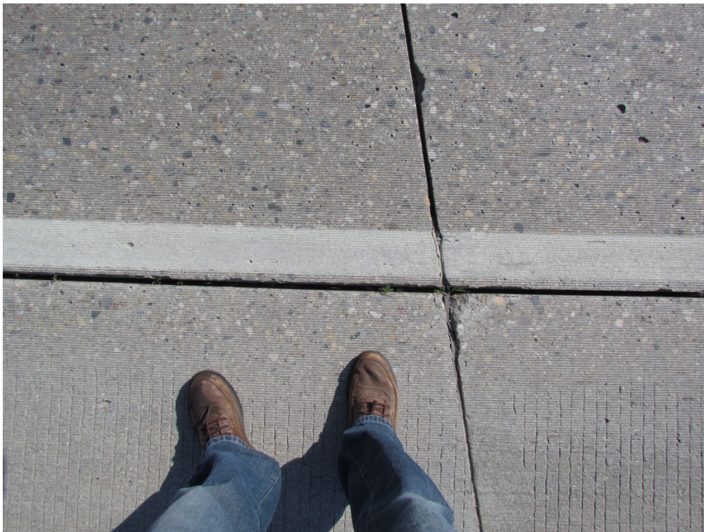
Segment 3B - SB White Surface applied Epoxy with 3M AW Elements – RP 147
