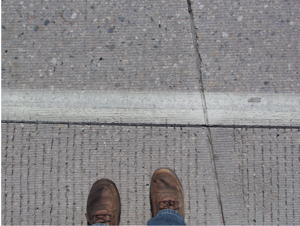
Segment 3A - SB White Surface applied Epoxy with Standard Glass Beads – RP 145
