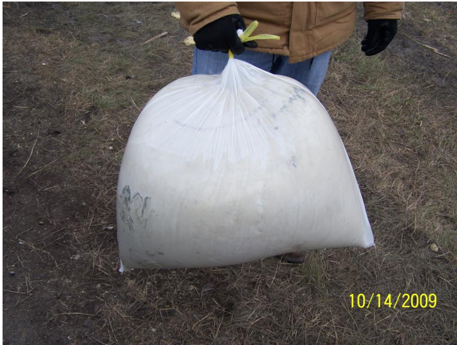
Photo 140: One half gallon of 985 Rigid Foam after expansion
