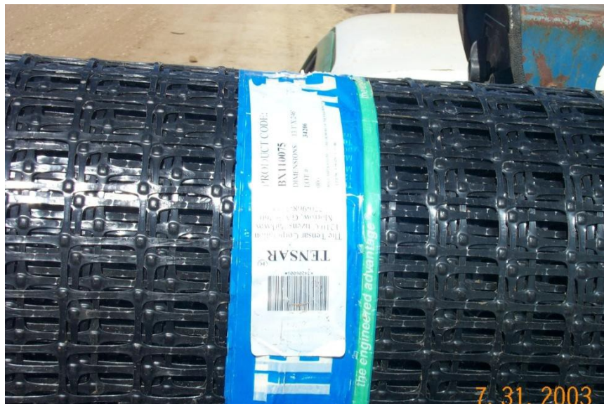
Photo 3 – A roll of Tensar Geogrid BX 1100.
