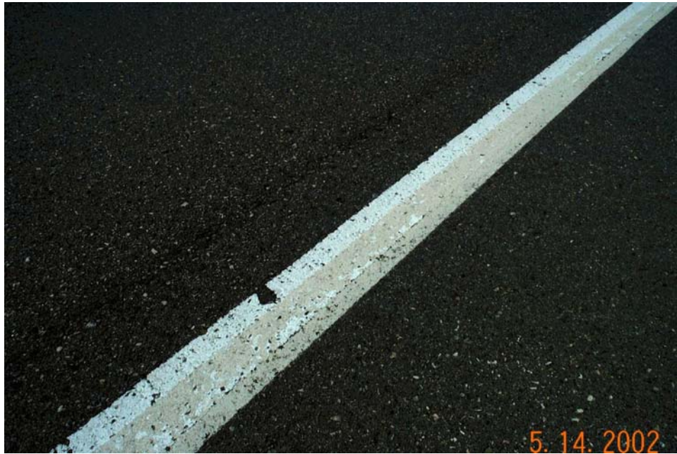
Photo 5 - Series 1200 remarked with water based paint.
