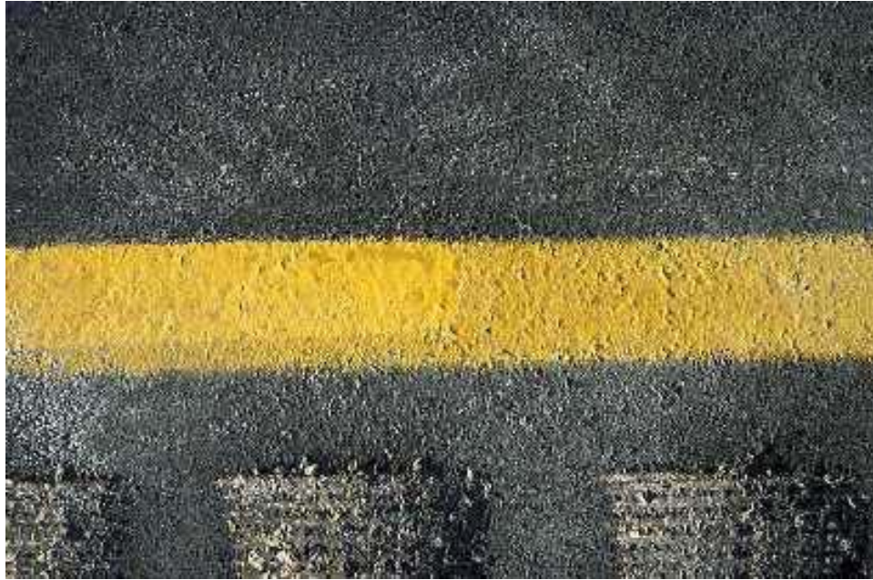
Photo 2 - Left half of photo is Series 1200 paint and the right half of photo is water based paint.
