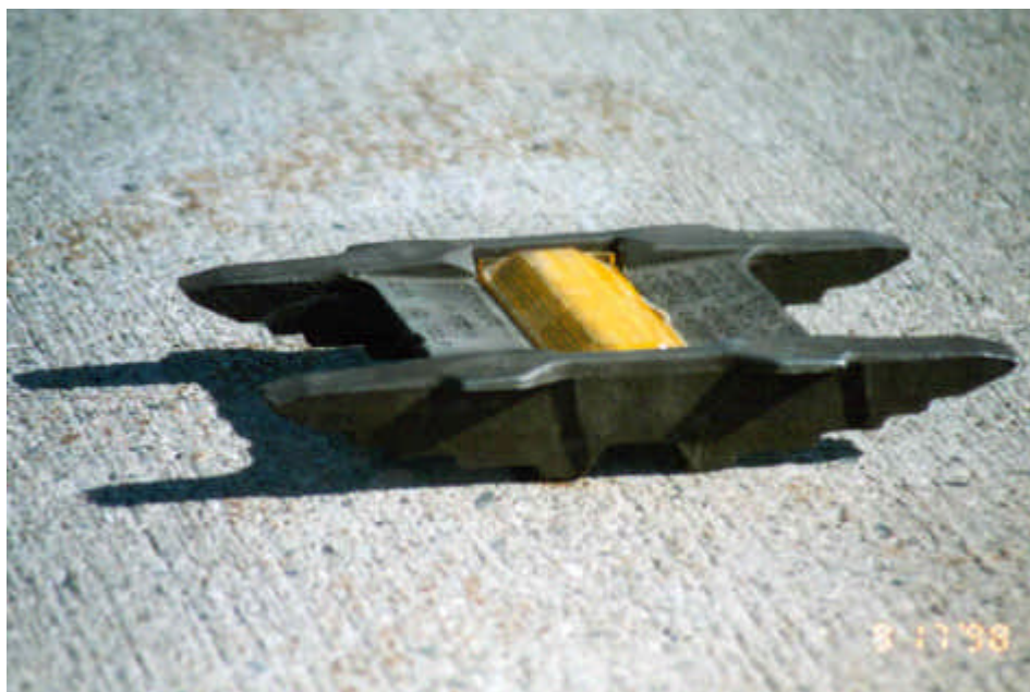
Photo 1- Stimsonite Lifelite 101 LP marker before installation.
