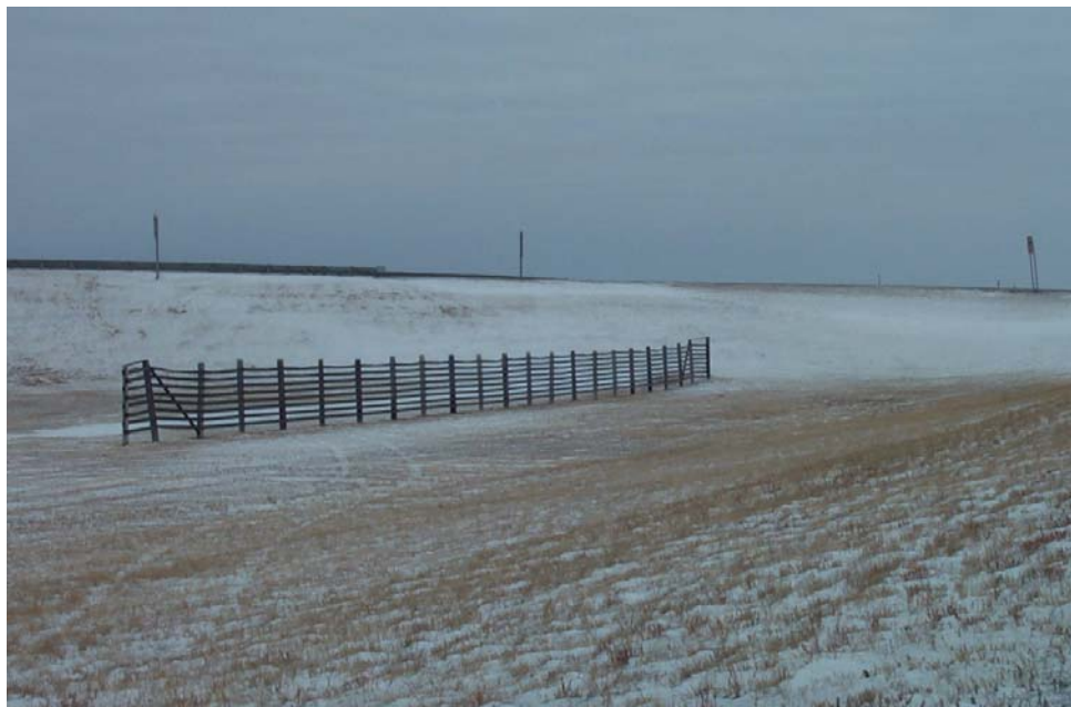
Photo 10 - A snow fence in at a low elevation at site 3 with relatively little snow accumulation.
