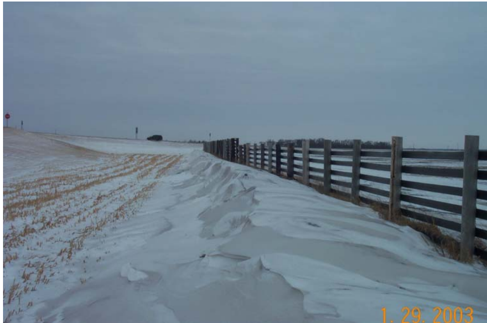
Photo 9 - A large drift accumulated by a snow fence at a relatively high location at site 3.
