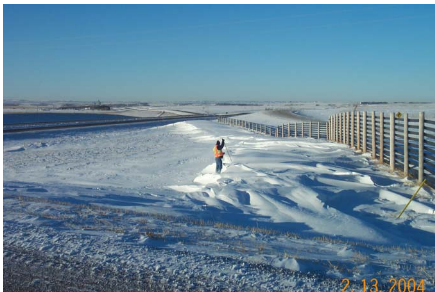
Photo 11 – Snow drift created by a fence at Site 2.
