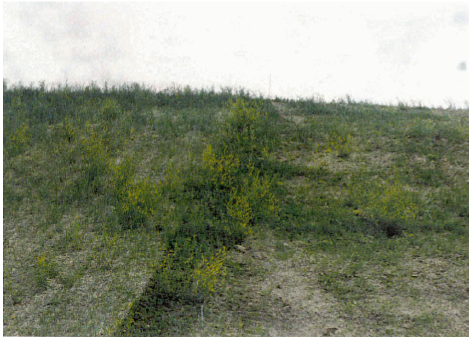
Photo - 13 A view from the bottom of the slope with the Double Netted Straw on the left, a narrow strip of uncovered soil in the center and the Soil Guard® on the right.
