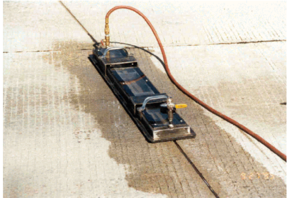
Photo 1. (IA-VAC) joint sealant tester
