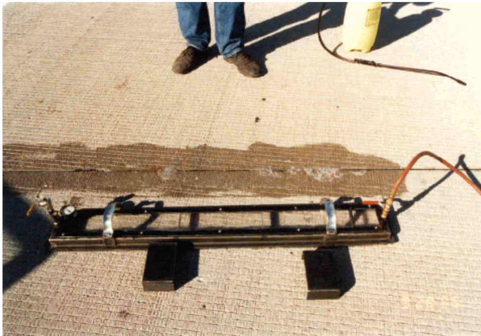
Photo 6. Leaks depicted after IA-VAC is removed
