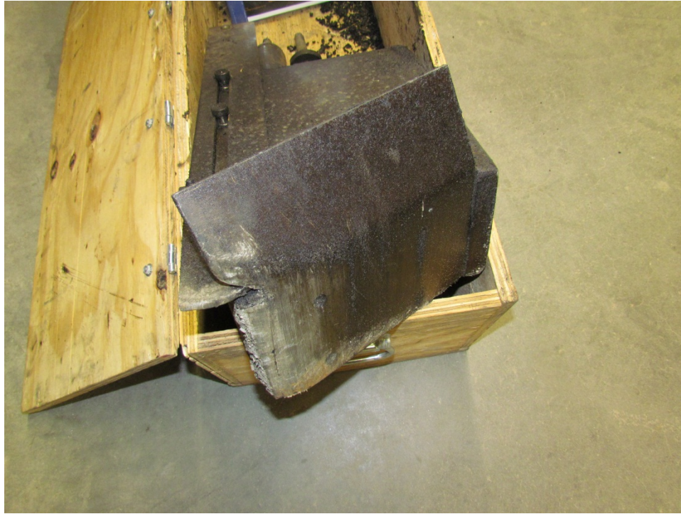
Photo 51: Ramp Champ shoe condition post construction.
