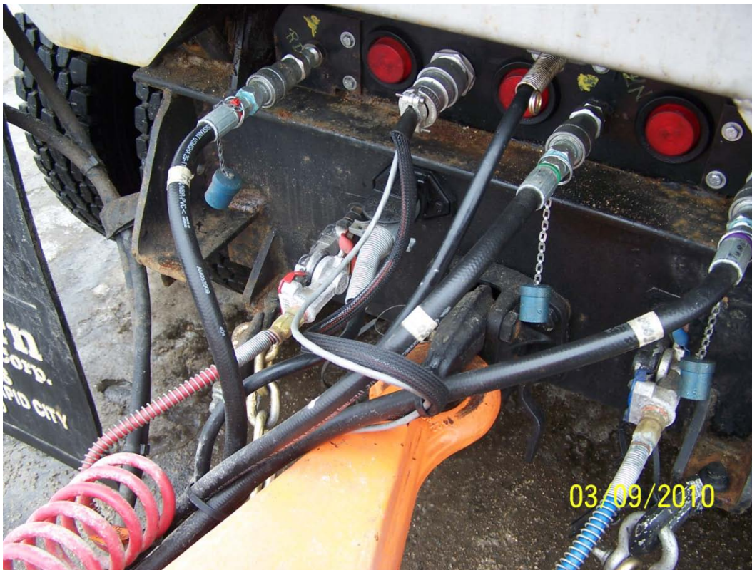
Photo 2 - Blue and red hoses broke during turning motions,
