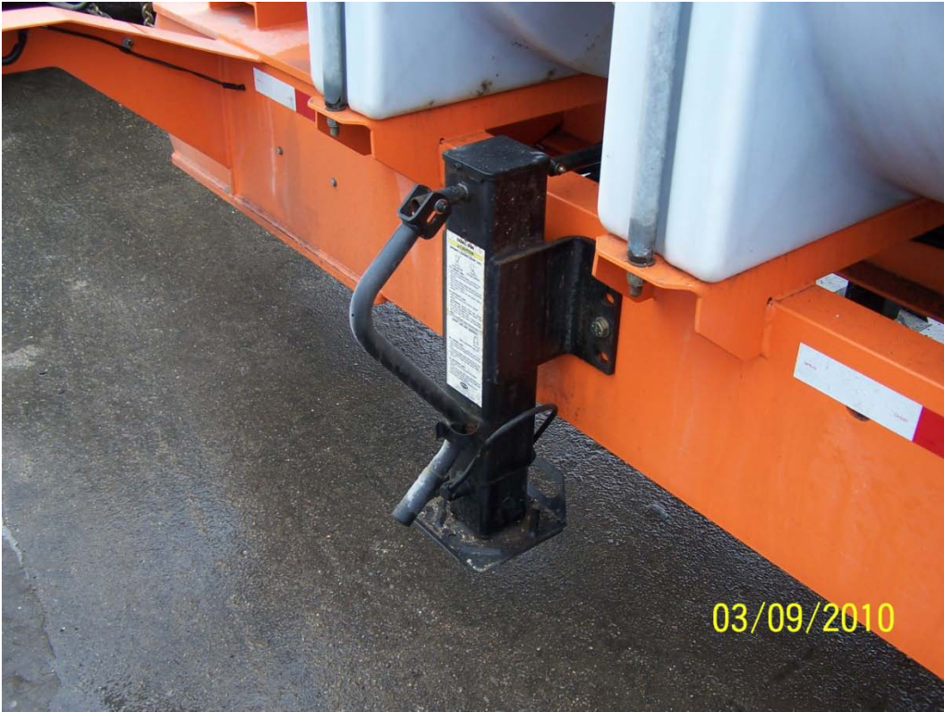
Photo 8 – Mechanical jack for the TowPLow.
