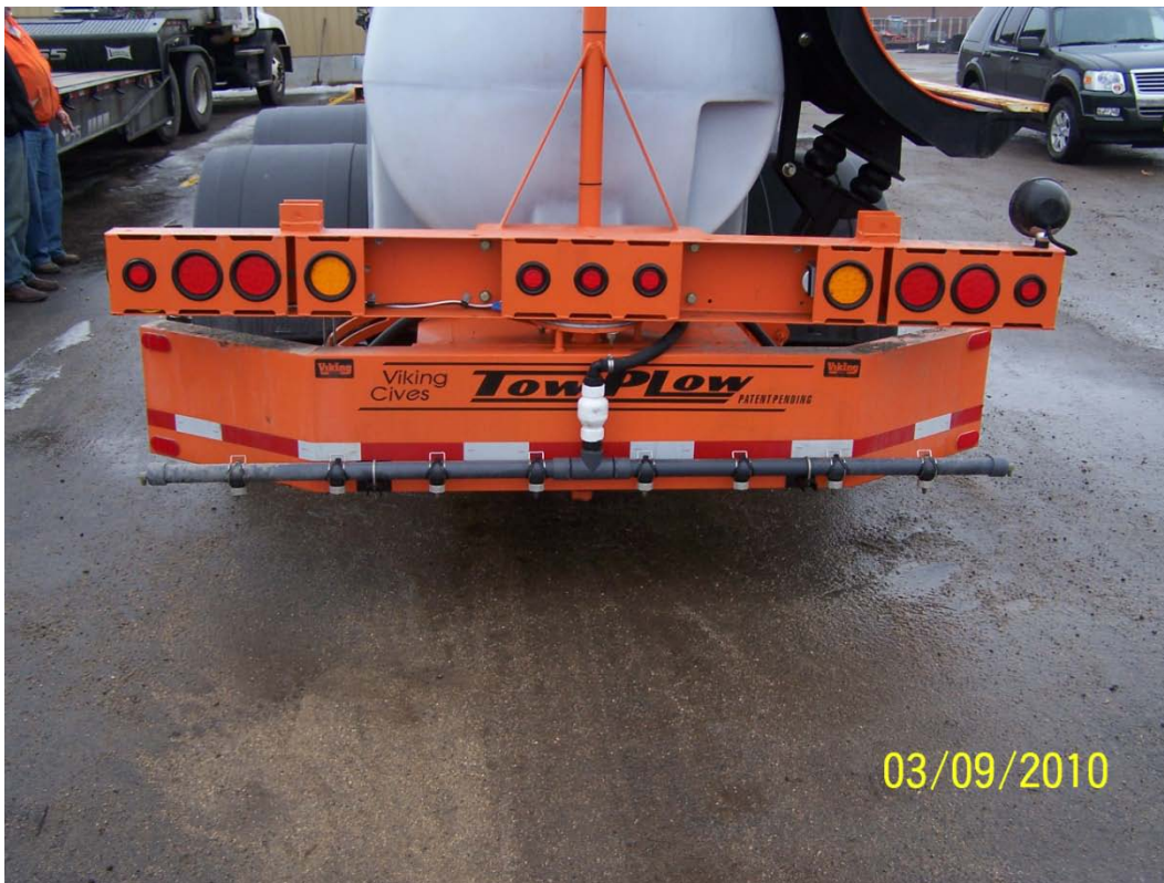
Photo 6 – Photo is displaying de-icing spray bar on the rear of TowPLow.
