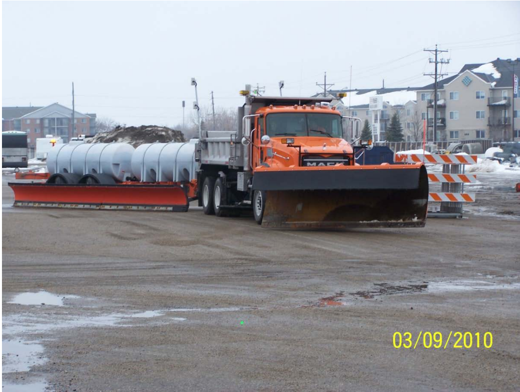
Photo 9 – Photo of the TowPLow fully deployed.
