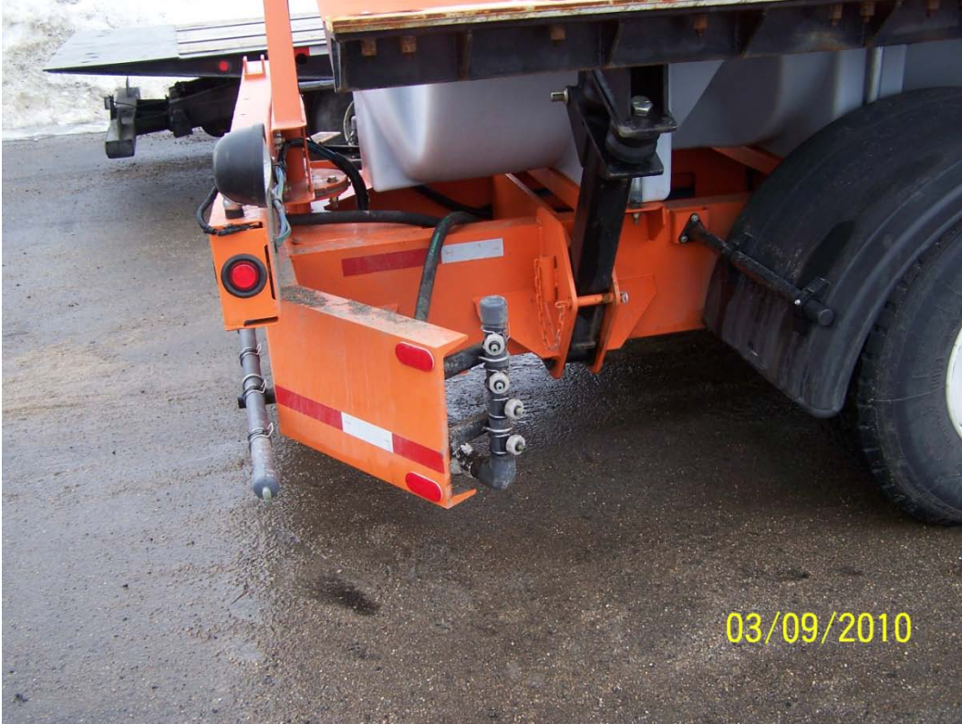
Photo 7 – Photo is displaying de-icing bar for adjacent lanes of roadway.
