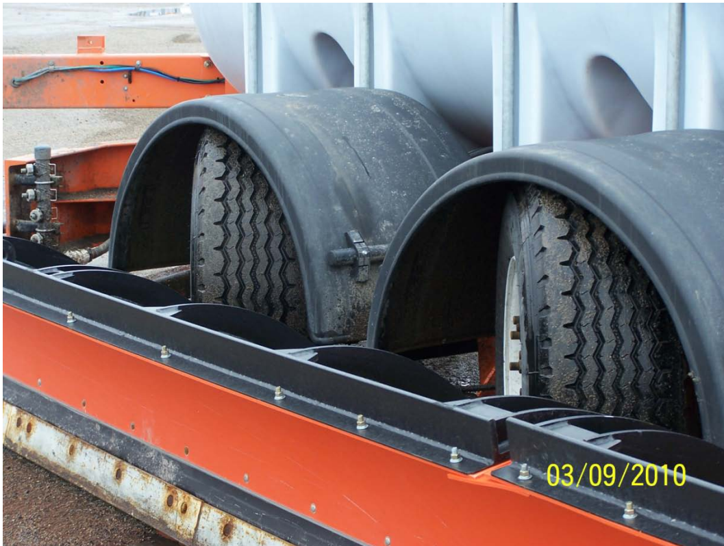
Photo 10 – Photo of TowPLow wheels rotated when fully deployed.
