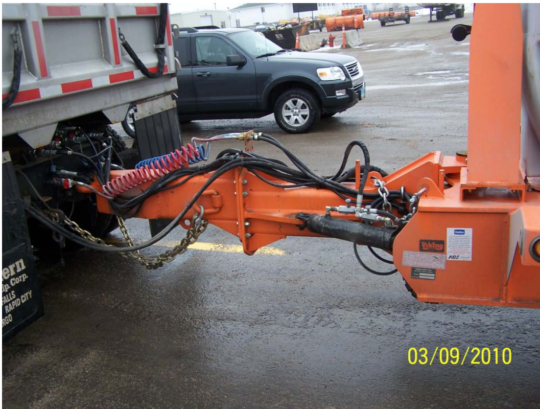
Photo 4 – Tongue of TowPLow attached to truck
