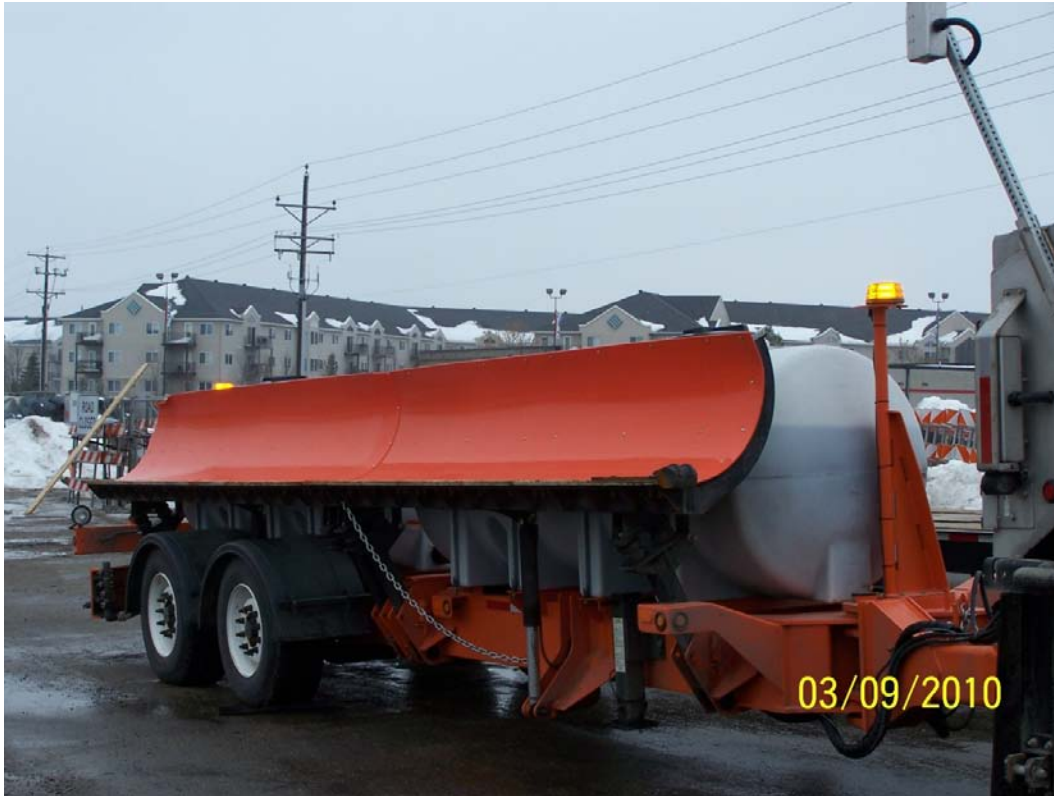
Photo 1 - An overview of TowPLow attached to vehicle
