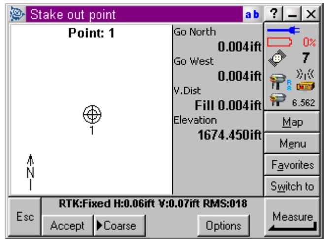
**Note:** Without a base station set-up, You can still navigate to a point, (ie. A control point that your not sure where it is). 1) Simply power on your Receiver, on the TSC2, 2) Select instrument, then 3) navigate to point. This should get you plus or minus 10M to the spot. (In this configuration, it acts just like a handheld GPS unit).
