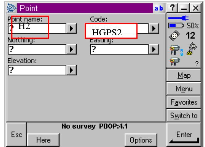
**NOTE:** When Using False Coordinates, Such as “You Are Here” you must put an “H” in front of the point number, and code. Ie. Point Name (H2), Code (HGPS2).
