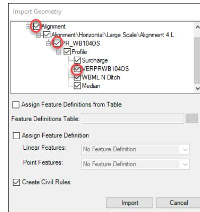
The alignments are imported without the applicable annotation group. Add alignment element annotation to assist with the review. This tool is in “OpenRoads Modeling (workflow) > Drawing Production (tab) > Annotations (panel) > Element Annotation > Annotate Element”. If multiple alignments are imported, they can all be annotated at once with the “All Elements in Model” option.
