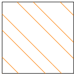
PERMEABLE TRENCH BACKFILL Cell Name = PERTRE Scale = 0.5 Row Spacing = 0.2 Column Spacing = 0 Angle = 135
