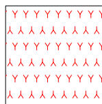
CLAY FILL Cell Name = CLAFIL Scale = 2.5 Row Spacing = 0 Column Spacing = 0 Angle = 0
