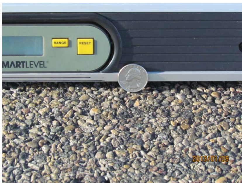
Photo 1: Rutting in a right wheel path in the driving lane of Segment 1.
