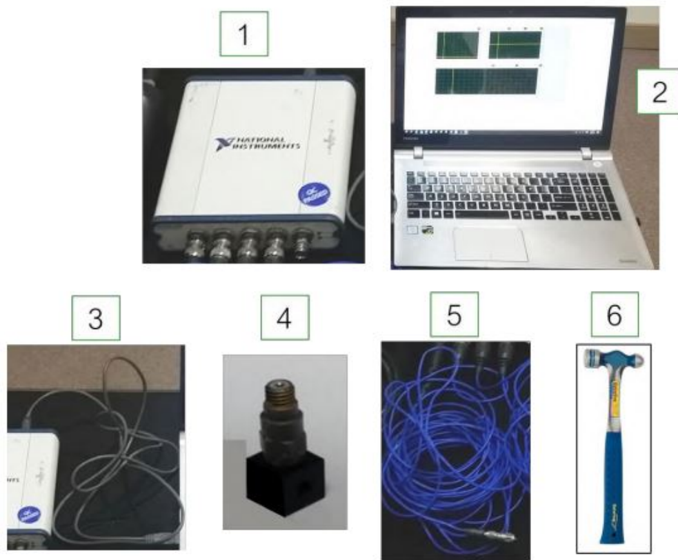
Figure 29.IE test equipment (1) NI-USB-4431 USB DAQ System. (2) Laptop w/ LabView software. (3) USB-A to USB-B Cable. (4) Accelerometer w/ mounting base. (5) Accelerometer BNC Cable. (6) Impact Hammer
