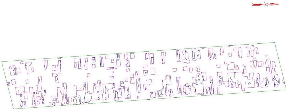
Figure 11. Bridge condition of Forest River South Bound.
