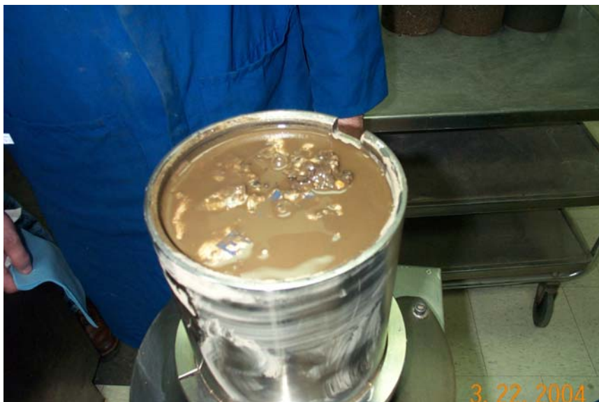
Photo 1 – Water on the surface of a gyratory compactor sample as it is being pushed out of the mold.
