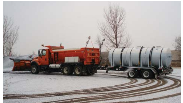
Typical anti-icing equipment.
