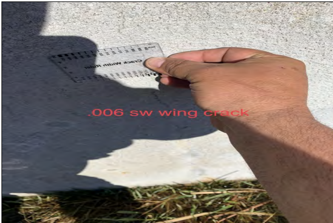
.006 SW wing crack
