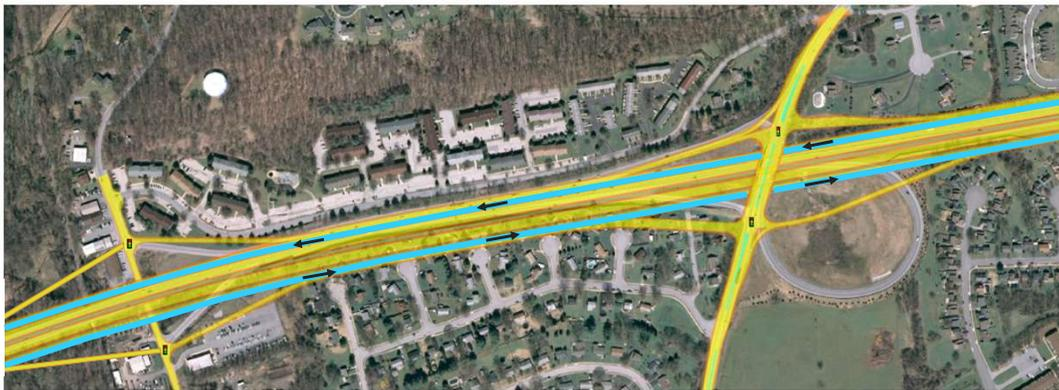
A simple, one-way Collector-Distributor Road on both sides of a freeway.
