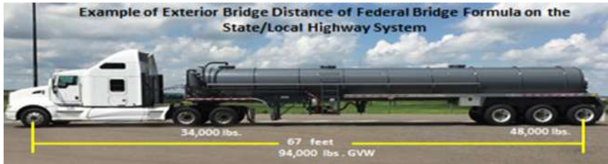
Figure 5: Illustration of Exterior Bridge Distance
