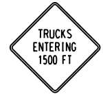
W8-54_1500FT TRUCKS ENTERING 1500 FEET
