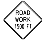
W20-1_1500FT ROAD WORK 1500 FT
