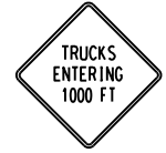
W8-54_1000FT TRUCKS ENTERING 1000 FEET
