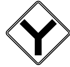
W2-5 Y INTERSECTION AHEAD
