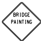
W21-50 BRIDGE PAINTING
