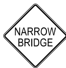
W5-2 NARROW BRIDGE
