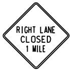
W20-5_RT_MILE RIGHT LANE CLOSED ONE MILE
