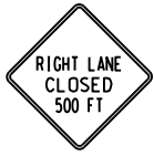
W20-5_RT_500FT RIGHT LANE CLOSED 500 FEET
