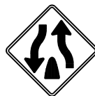
W6-2 END DIVIDED HIGHWAY
