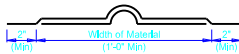
Fabric waterproofing shall be applied in accordance with Section 740 of the NDDOT Specifications. All material and work shall be included in the pay item "Class AE-3 Concrete." FABRIC WATERPROOFING DETAIL
