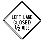
W20-5_LT_HLF MILE LEFT LANE CLOSED HALF MILE
