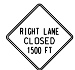
W20-5_RT_1500FT RIGHT LANE CLOSED 1500 FEET
