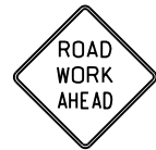
W20-1_AHD ROAD WORK AHEAD
