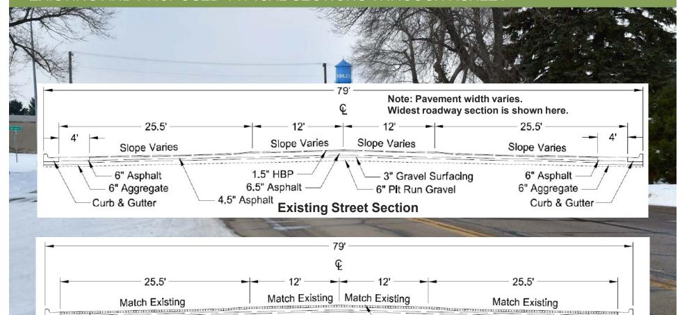
Through the City of Ashley, the top of the pavement will be removed by milling, and an equal thickness of new asphalt pavement will replace the removed pavement.
