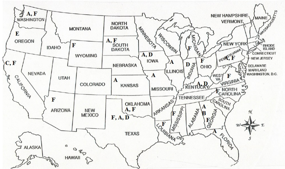
Fig. 1. Slab stabilization materials used throughout U.S. ((A: pozzolan cement, D: limestone dust cement, C: cement only, A:Asphalt cement only, E: sand cement, F: high density polyurethane, adopted from ACPA)
