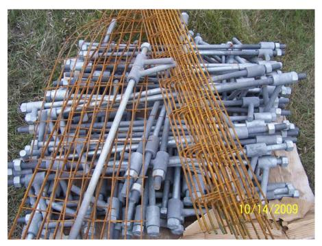
**Photo 141: Internal Joint Ties**
