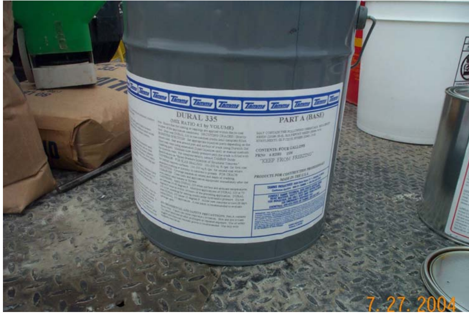
Photo 16 - Resin or base component of the Tamms Dural 335 sealer.
