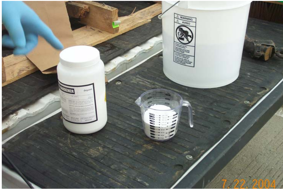
Photo 9 - Hardener that is added to the resin of Degusa Degadeck Crack Sealer.
