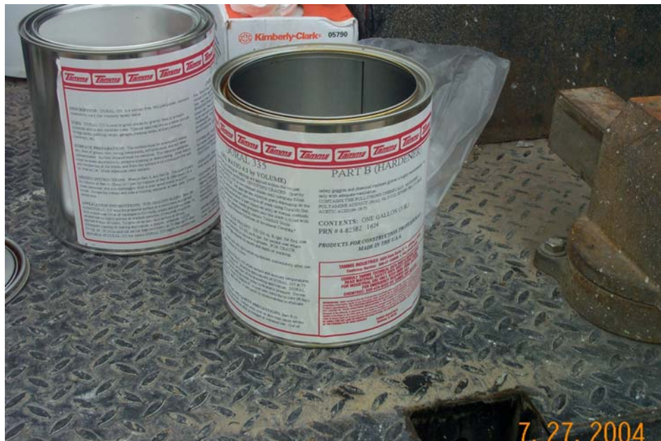
Photo 15 - Hardener that is added to the Tamms Dural 335 resin.
