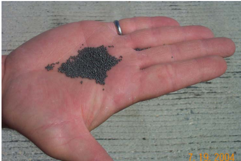
Photo 4 - Size of shot used in shotblasting.
