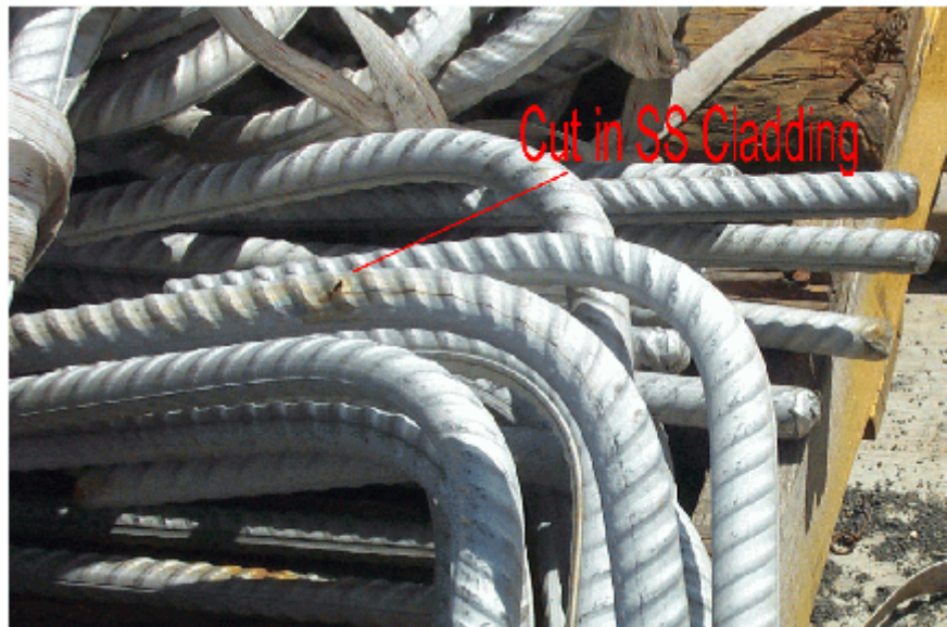
Photo 3. Cut in Stainless Steel Cladding
