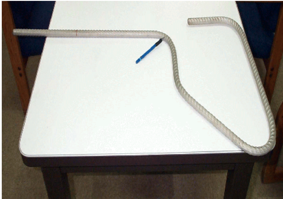
Photo 1. Example of Stainless Steel Clad Rebar
