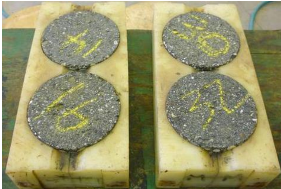
Figure 2: Placing Specimens in the Molds for an APA Run
