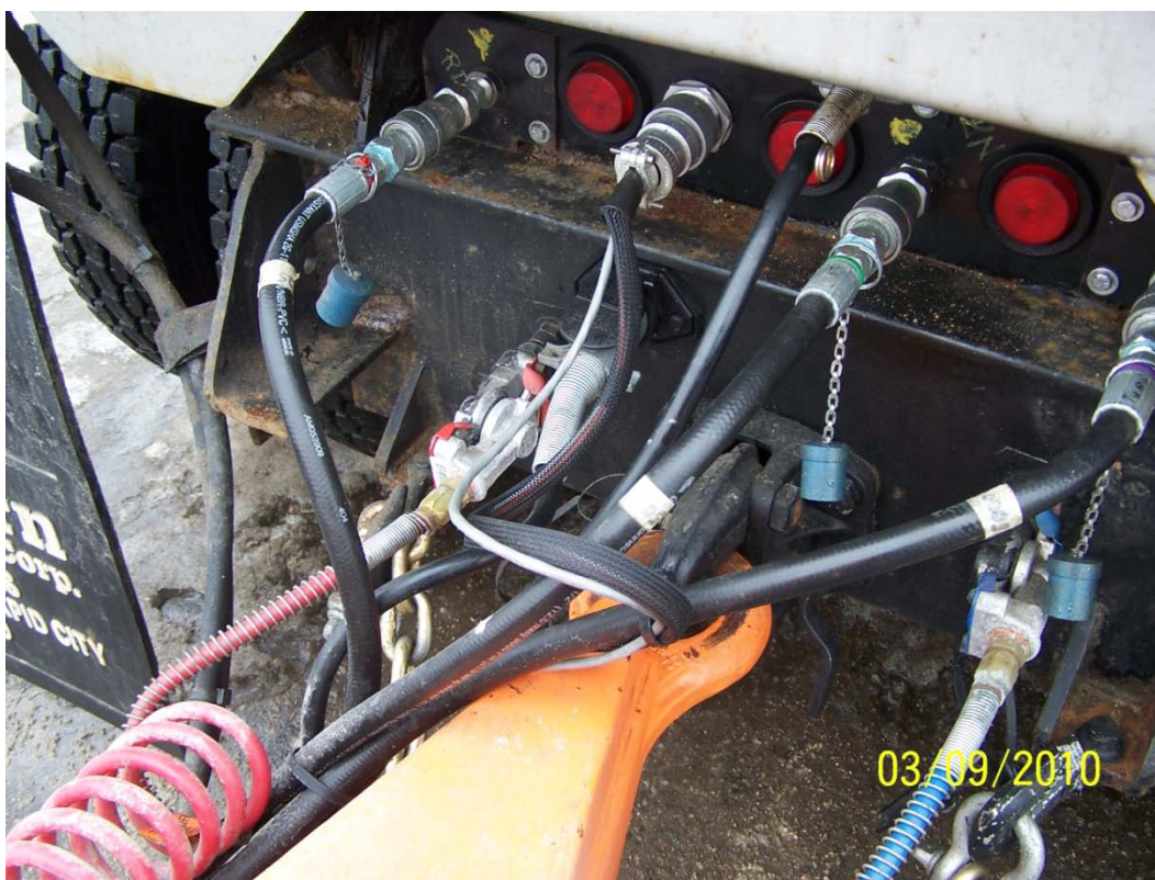
Photo 2 - Blue and red hoses broke during turning motions,
