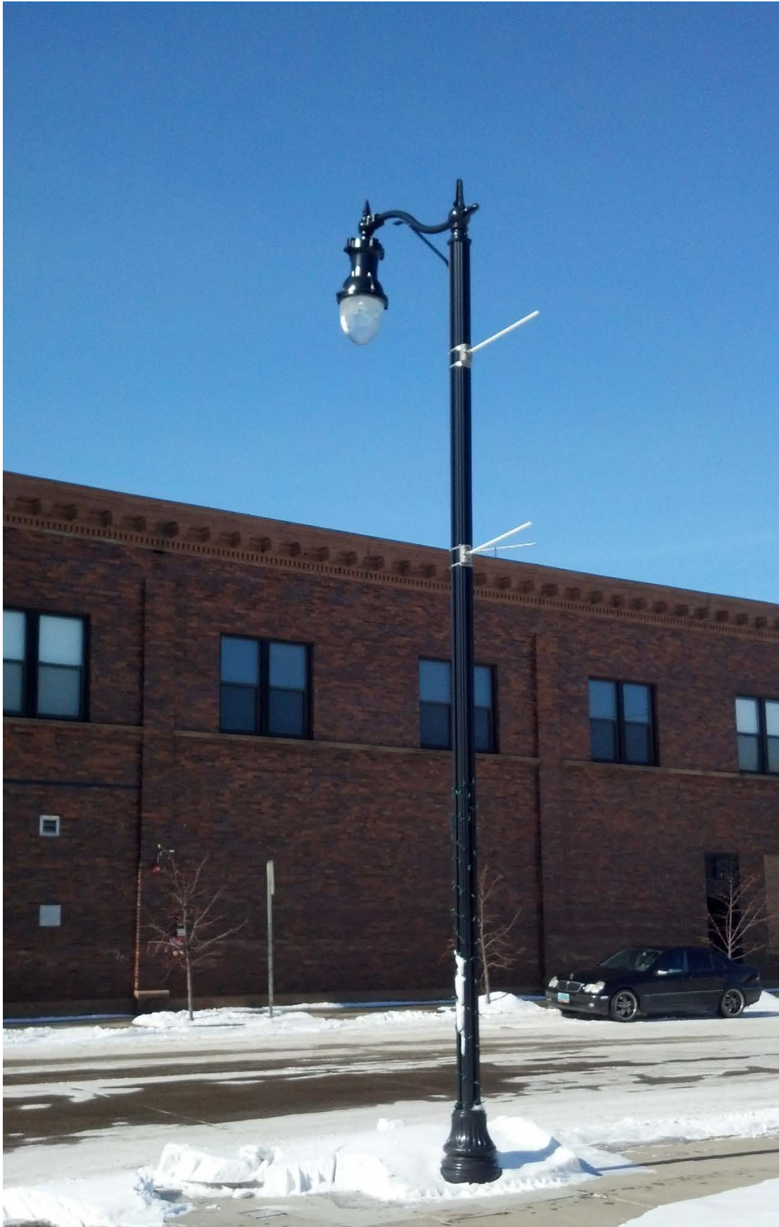
Figure 9: Taller style Holophane hanging light. The city has installed 4 poles of differing heights and styles like these over the past two year on Sims Street between Villard and 1 st St. We have received positive feedback from the community. These luminaires are also LED, providing modern efficiency with the warm look of a period correct light that matches the era of the buildings.
